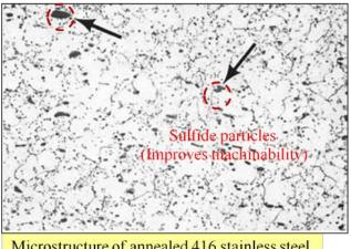
Microstructure of annealed 416 stainless steel etched with Vilella's reagant
