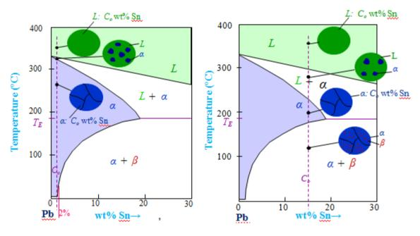
☐ To reiterate an important point: Phase diagram do not contain microstructural information (i.e. they cannot tell you what the microstructures produced by cooling is. Often microstructural information is overlaid on phase diagram for convenience. Hence, strictly cooling is not in the domain of phase diagram – but we can overlay such information keeping in view the assumptions involved.
