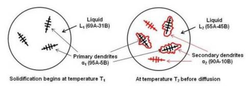
Schematic Representation of the Alloy 70A-30B at Temperatures T<sub>1</sub> and T<sub>2</sub>
