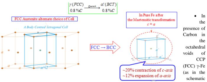
below)  $\rightarrow$  the contraction along the c-axis is impeded by the carbon atoms. (Note that only a fraction of the octahedral voids are filled with carbon as the percentage of C in Fe is small).
