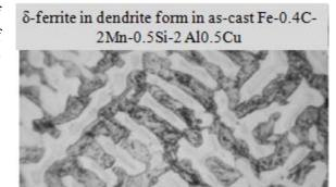
body higher limit of The 1539°C. • This is not stable at room temperature in plain carbon steel. However it can be present at room temperature in alloy steel especially duplex stainless steel.
