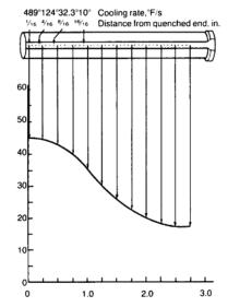
Fig. 4.4 Method of plotting hardness data from an end-quenched Jominy specimen.
