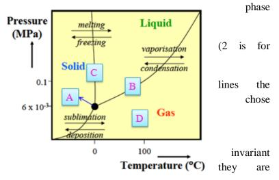
• The single phase region at point D, T and P can both be varied while still being in the single phase region with F = 2.
