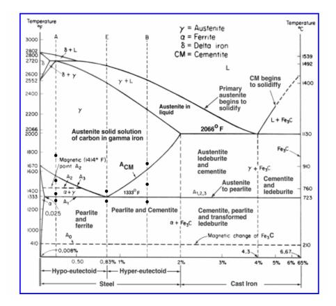
**Figure: Iron – Cementite Phase Diagram**
