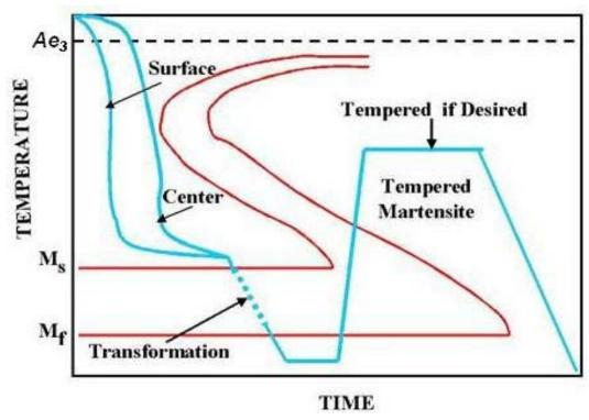
Fig. 4. 7. Schematic representation of the Martempering process.
