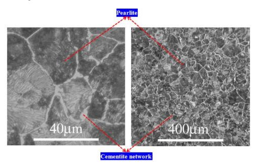
Application of Lever rule in Fe-Fe<sub>3</sub>C phase diagram
