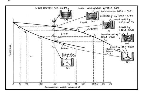
Figure: The above figure represents the very slow cooling, under equilibrium conditions, of a particular alloy 70A-30B will now be studied to observe the phase changes that occur
