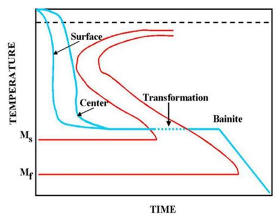
Fig. 4.8. Schematic representation of the Martempering process.
