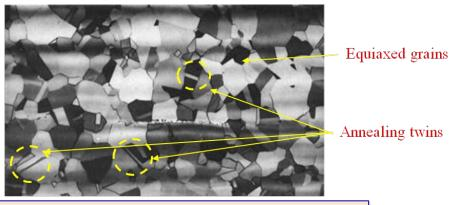
Microstructure of annealed type 316L austenitic stainless steel etched in 20% HCl, 2% NH4FHF, 0.8% PMP
