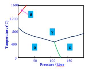
• The above figure represents the phase diagram for pure iron. The triple point temperature and pressure are 490°C and 110 kbars, respectively.  $\alpha$ ,  $\gamma$  and  $\epsilon$  refer to ferrite, austenite and  $\epsilon$ -iron, respectively.  $\delta$  is simply the higher temperature designation of  $\alpha$ .
