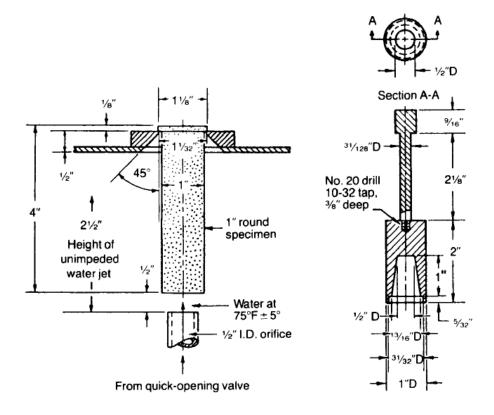
Fig. 4.3 Jominy-Boegehold specimen for end-quench test for hardenability.
