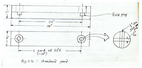
One yard is then defined as the distance between 2 central transverse lines of the gold plug at 62 f. the purpose of keeping the gold plug lines at neutral axis is that due to bending of beam the neutral plane remains unaffected, secondly the plug being in the well is protected from accidental damage. The supports of the yard bar should be at such distance the 2 end faces of the bar are at zero slopes.
