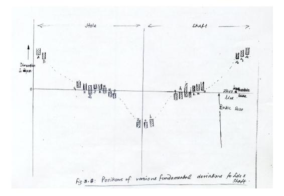
fig 3.8 positions of various fundamental deviations for hole & shaft
