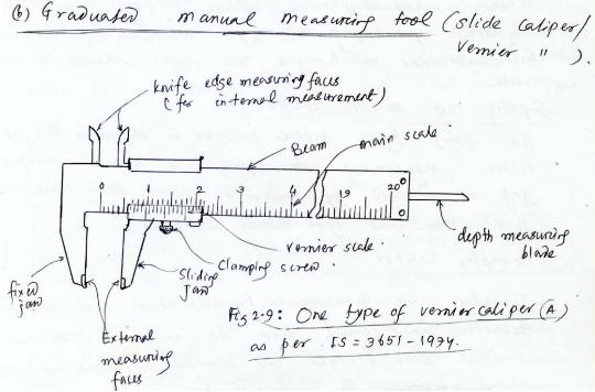
300,0-500,0-750,0-1000,750-1500 and 1500-2000mm. out of 3 types (A,B,C) only A type is shown in fig 2.9.
