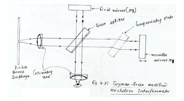
In this way all rays are reared parallel to the central rays and thus all rays describe the same path. All modern two beam interferometer are based on the arrangement. The mirror m,m are arranged to the optical axis. If mirror m is kept fixed and m is moved slowly exactly to itself the observe evil note periodic change in the intensity of the field being viewed from bright to dark for every movement of mirror in fact the intensity variation is found to be sinusoidal.
