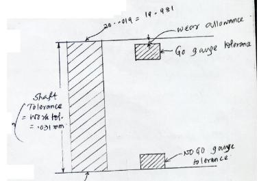
(i)size of Go snap gauges =19.9810-.00031 =19.9807mm- higher limit and 19.9807-.0031=19.9876mm- lowest limit
