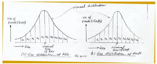
An automatic gauge can segregate them into 10 different groups (with 0.01mm limit) for selective assembly of a group of shaft with corresponding group of hole (say with HG) thus parts with tolerance of 0.001mm are obtained due to grouping and both the condition.
