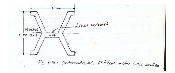
has 2 fine lines engraved over it. It is in oxidisable and can have a good finish required for ruling good quality lines. The bar is kept at 0 c and under normal atmospheric pressure.
