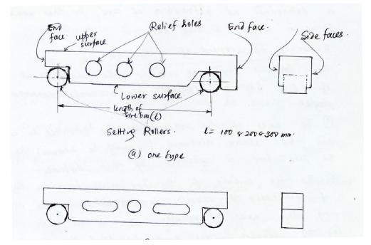
It consists of a steel bar and rollers. The sine bars are available in several designs for different applications. Two most common types are shown in fig 2.18.
