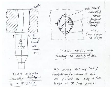
Similarly a NOGO gauge with circular section can't check the availability of the hole as shown in fig 3.13. here a pin type shape is appropriate which can check both circularity and size of hole.
