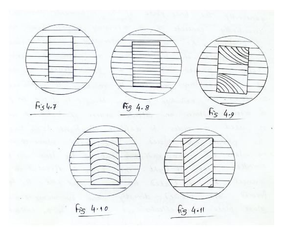
In case taper is present in some other direction i.e surface of the gauge is inclined to the base plate at some other angle then the fringe pattern will be as shown in fig 4.9.
