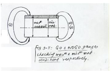
(iii) Go gauges should check all the related dimensions simultaneously whereas
