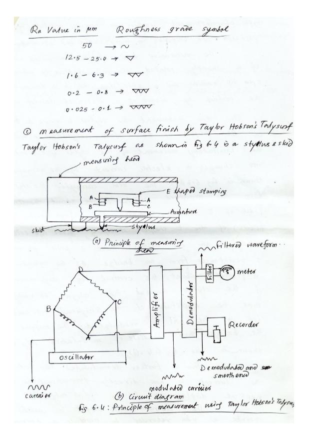
type of instrument working on carrier modulating principle. Its response in more rapid and accurate.
