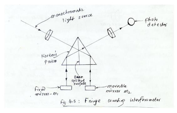
These are used to measure linear mechanical motion directly in terms of wave length of light. Every motion of x/2 amount by moving mirror will move the parallel fringes by one fringe. This can be counted by eye or with hole detector.
