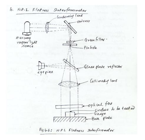
This instrument is mainly used for checking the flatness of flat surface. This interferometer was designed by national physical laboratory and is commercially manufactured by Higher and Wats Ltd.
