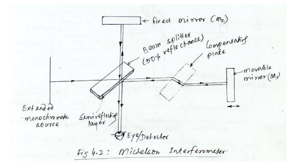
Each half wavelength of mirror travel produces a change in the measured optical path of one wavelength and the reflected beam from the moving mirror shifts through 360 phase change. When the reference beam reflected from fixed mirror and the beam reflected from moving mirror rejoin at the beam splitter, they alternately rein force and cancel each other as the mirror moves. Thus each cycle of intensity at the eye represents distance of mirror travel.
