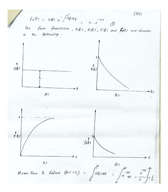
The constant hazard model assumes that ports don't deteriorate with time. This model is also called exponential reliability case.
