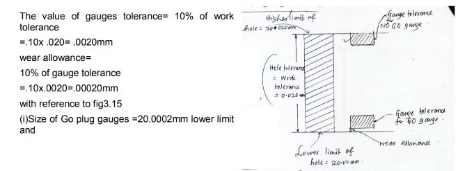
20.0002+.002=20.0022mm-higher limit (ii)Size of NOGO plug gauges 20.020-20,020-.002= 20.018 lower limit
