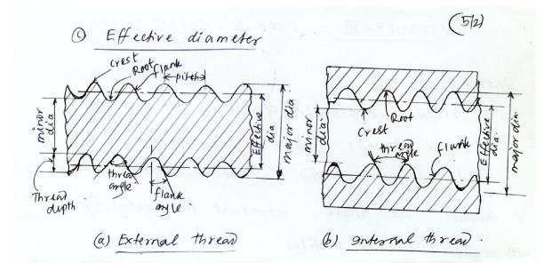
Fig 5.2 Basic nomenclature of external i internal thread.
