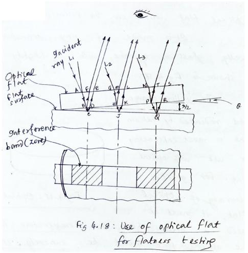
The behavior of a ray of light as it passes through the optical flat to the surface and thence to the observes eye may be understood as follows
