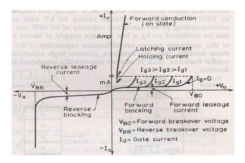
$V_{BO}$ =Forward breakover voltage
