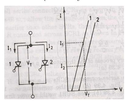
For equal sharing of current, SCRs must have same V-Icharacteristics during forward conduction.  $V_T$  across them must be same. For same  $V_T$ , SCR 1 share  $I_I$  and SCR 2 share  $I_2$ .
