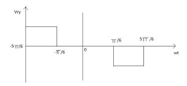
If we go for harmonic analysis  $V_{RY=\sum_{n=1,3,5}^\infty \frac{4V}{n\pi}} \sin \frac{n\pi}{3} \sin n \left(\omega t + \frac{\pi}{6}\right)$
