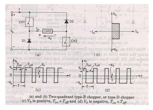
When CH1 and CH2 both are on then  $V_0=V_s$ .
