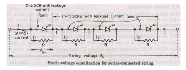
Let SCR1 has lower leakage current  $I_{bmn}$ , It will block a voltage comparatively larger than other SCRs.
