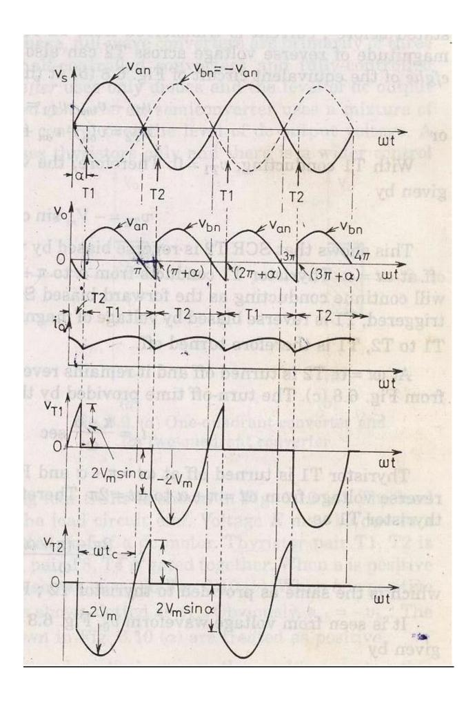
$$V_0 = \frac{1}{\pi} \int_{\alpha}^{\pi+\alpha} V_m \sin(\omega t) d(\omega t)$$
