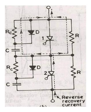
SCR 1 has short recovery time as compared to SCR 2.  $\Delta_Q$  is the difference in reverse recovery charges of two SCR 1 and SCR 2. Now we assume the SCR 1 recovers fast . i.e it goes into blocking state so charge  $\Delta_Q$  can pass through C . The voltage induced by  $c_1$  is  $\Delta_Q/C$ , where is no voltage induced across  $C_2$ .
