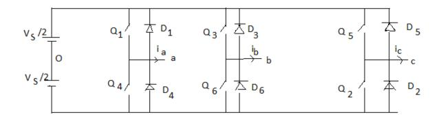
When  $Q_1$  is switched on, terminal a is connected to the positive terminal of dc input voltage.
