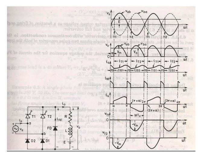
$$V_0 = \frac{1}{\pi} \int_{\alpha}^{\pi} V_m \sin(\omega t) d(\omega t)$$
