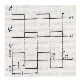
$$V_o(rms) = \frac{1}{T_0/2} \int_0^{T_0/2} \frac{V_S^2}{4} dt = \frac{V_S}{2}$$
