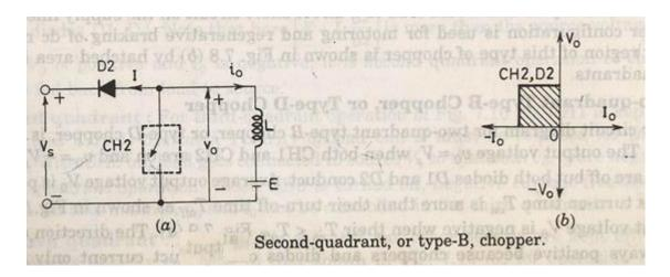
When switch are closed the load voltage E drives current through L and switch. During  $^{T_{\mathit{on}}}$
