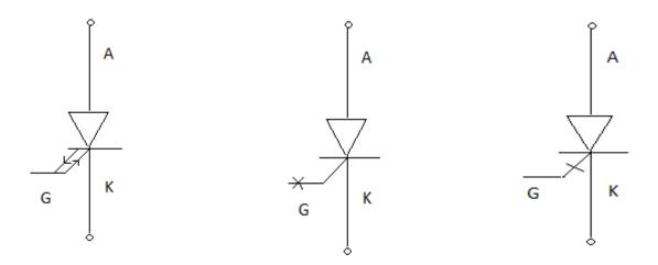
Conventional SCR are turned on by a positive gate signal but once the SCR is turned on gate loses control over it. So to turn it off we require external commutation circuit. These commutation circuits are bulky and costly. So due to these drawbacks GTO comes into existence.
