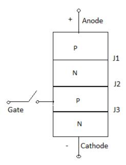
A forward voltage is applied between anode and cathode with gate circuit open.
