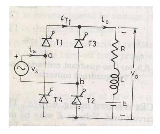
$$V_0 = \frac{1}{\pi} \int_{\alpha}^{\pi+\beta} V_m \sin(\omega t) d(\omega t)$$
