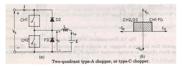
Both the switches never switch ON simultaneously as it lead direct short circuit of the supply.
