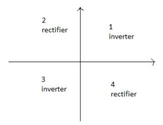
During interval 1  $v_0$  and  $i_0$  both are positive
