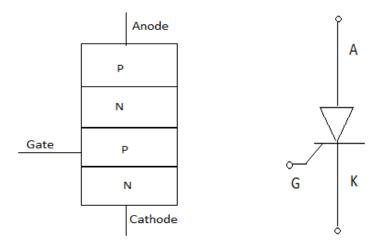
SCR is made up of silicon, it act as a rectifier; it has very low resistance in the forward direction and high resistance in the reverse direction. It is a unidirectional device.
