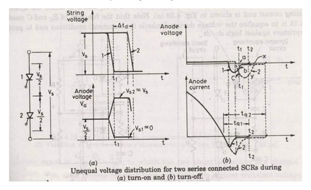
SCR 1 and SCR 2 have different dynamic characteristics. Turn ON time of SCR 2 is more than SCR 1 by time  $\Delta t_d$ .
