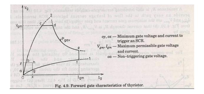
$V_q$  = +ve gate to cathode voltage.
