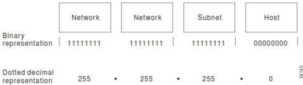
Subnet mask bits should come from the high-order (left-most) bits of the host field, as Figure 30-8 illustrates. Details of Class B and C subnet mask types follow. Class A addresses are not discussed in this chapter because they generally are subnetted on an 8-bit boundary.
