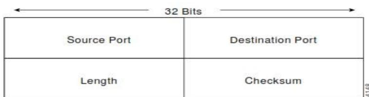
Source and destination ports contain the 16-bit UDP protocol port numbers used to demultiplex datagrams for receiving application-layer processes. A length field specifies the length of the UDP header and data. Checksum provides an (optional) integrity check on the UDP header and data.
