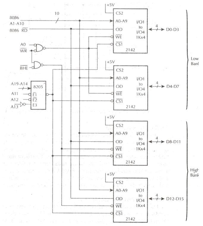
FIGURE 3.5.5 – 2K \* 8 STATIC ARRAY WITH A0 and BHE AS DIRECT CHIP SELECT INPUTS
