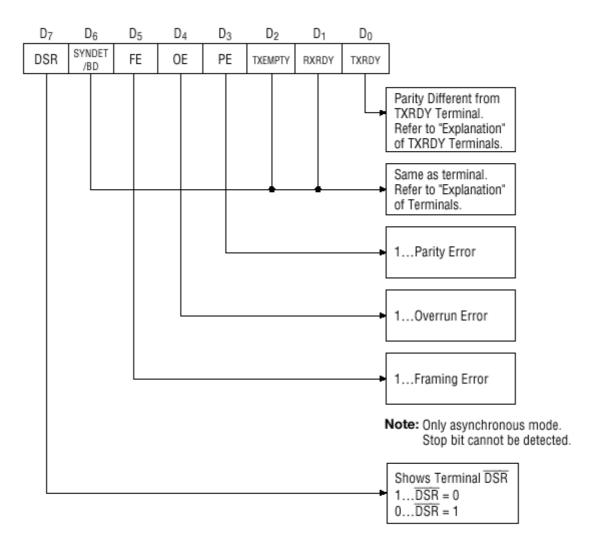
Fig. 5 Bit Configuration of Status Word
