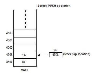
Figure.29 The PUSH operation of the Stack
