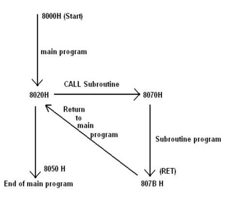
Fig.33 Diagrammatic representation of subroutine program execution
