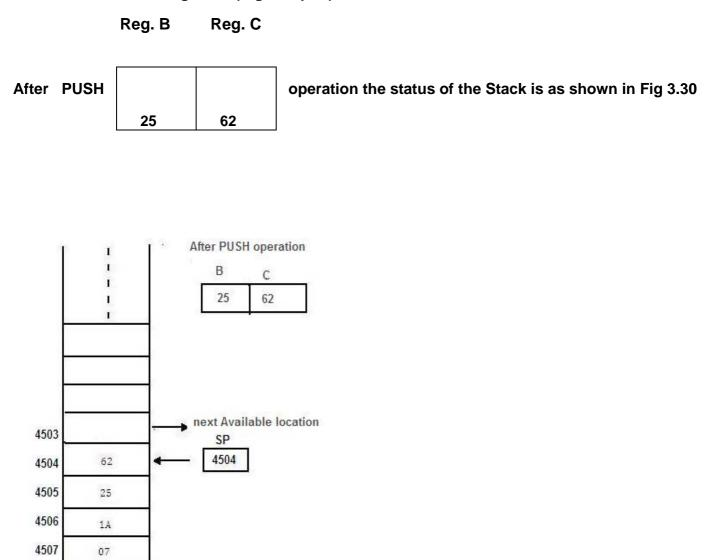
Figure .30 After PUSH operation the status of the stack
