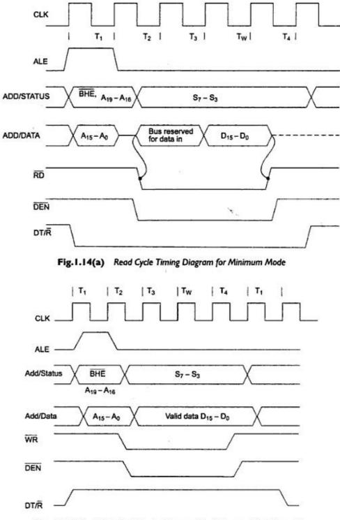
Fig. 1.14(b) Write Cycle Timing Diagram for Minimum Mode Operation
