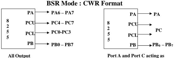
Port A and Port C acting as O/P. Port B acting as I/P
