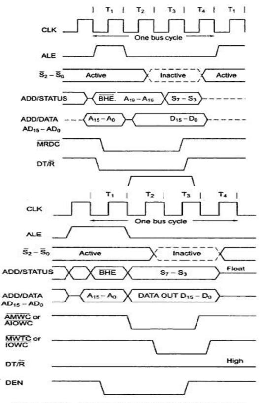
Fig. 1.16(b) Memory Write Timing in Maximum Mode
