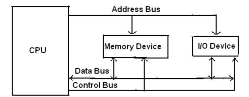
Fig.1 Block diagram of a Microcomputer
