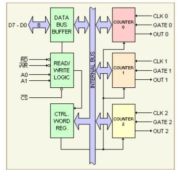
Fig: Block diagram of an 8253 programmable interval timer
