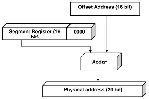
Figure 1 Fig: Physical address calculation
