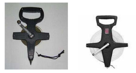
This may be 30m, 50m or 100m long and 13mm wide. It has handles similar to those on the chain and is wound on a steel cross. It is more accurate but less robust than the chain. The operating tension and temperature for which it was graduated should be indicated on the band.
