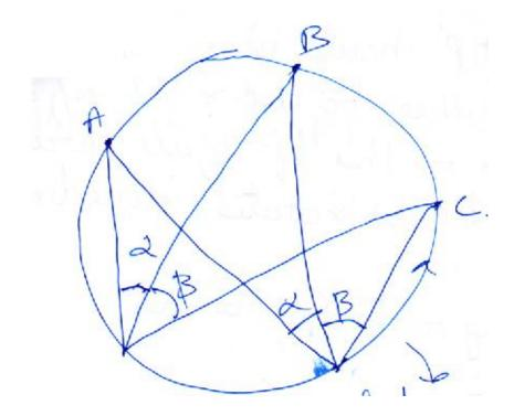
Indeterminate solution if point occupied at the circum circle of the three control points :-
