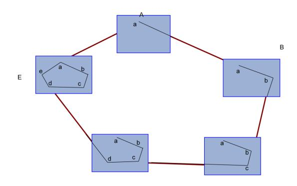
Plane Tabling using Traversing Method
