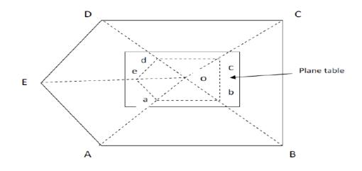
Plane Tabling using Radiation Method
