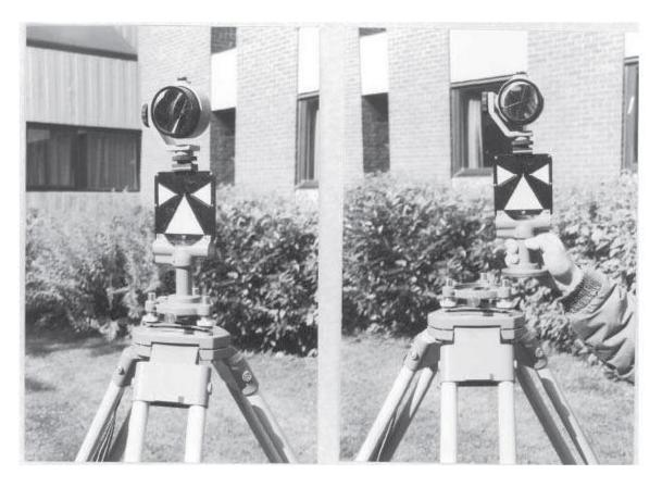
*Figure13.1.* Interchangeable target and tribrach
