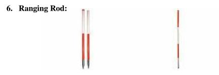
These are poles of circular section 2m, 2.5m or 3m long, painted with characteristic red and white bands which are usually 0.5m long and tipped with a pointed steel shoe to enable them to be driven into the ground. They are used in the measurement of lines with the tape, and for marking any points which need to be seen.
