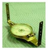
This consists of two pairs of vanes set at right angle to each other with a wide and narrow slit in each vane. The instrument is mounted upon a pole, so that when it is set up it is at normal eye level. It is also used for setting out lines at right angle to the main chain line.
