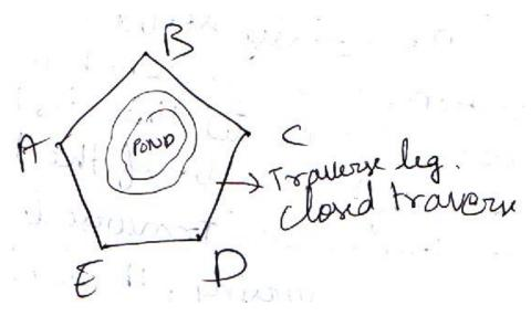
Fig 2.1 (a) Closed traverse is suitable for the survey of boundaries of ponds, forests etc.
