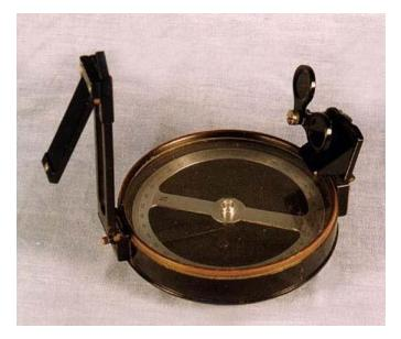
This is an instrument used for the measurement of magnetic bearings. It is small and portable usually carried on the hand. This Prismatic Compass is one of the two main kinds of magnetic compasses included in the collection for the purpose of measuring magnetic bearings, with the other being the Surveyor's Compass. The main difference between the two instruments is that the surveyor's compass is usually larger and more accurate instrument, and is generally used on a stand or tripod.
