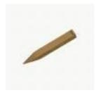
Pegs are made of wood 50mm x 50mm and some convenient length. They are used for points which are required to be permanently marked, such as intersection points of survey lines. Pegs are driven with a mallet and nails are set in the tops.
