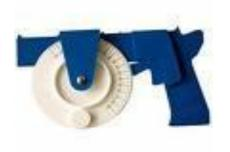
This instrument is generally used to obtain roughly the slope angle of the ground. It consists of a rectangular, telescopic tube (without lenses) about 125mm long with a graduated arc attached. A small bubble is fixed to the vernier arm, once the image of the bubble is seen reflected in the eyepiece the angle of the line of sight can be read off with the aid of the reading glass.
