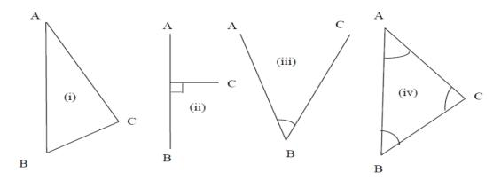
Fig. 6.1: Fixing the third points using two points
