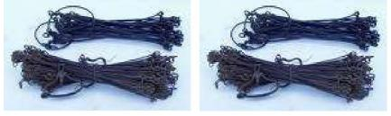
Chains are made up of links which measure <u>200mm</u> from centre to centre of each middle connecting ring and surveying brass handless are fitted at each end. Tally markers made of plastic or brass are attached at every whole metre position or at each tenth link. To avoid confusion in reading, chains are marked similarly form both end (E.g. Tally for 2m and 18m is the same) so that measurements may be commenced with either end of the chain
