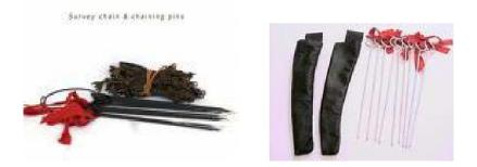
Arrow consists of a piece of steel wire about 0.5m long, and are used for marking temporary stations. A piece of coloured cloth, white or red ribbon is usually attached or tied to the end of the arrow to be clearly seen on the field.
