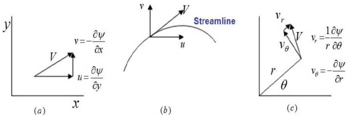
Fig. Velocity components along a streamline
