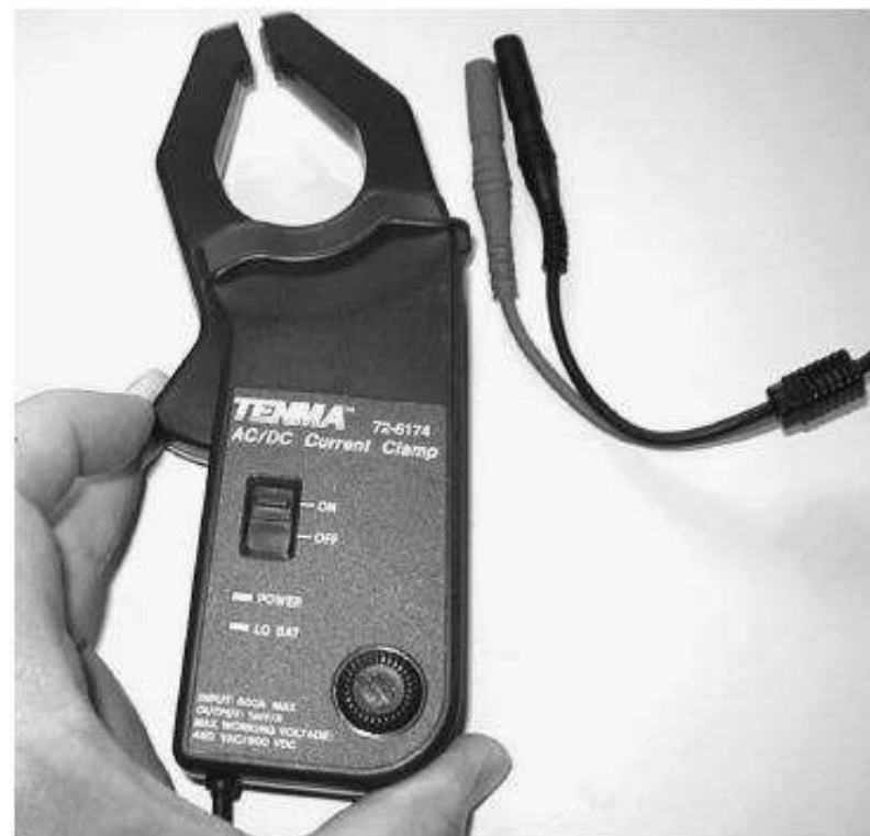
FIGURE: An AC and DC current clamp such as the one shown can be used with a regular digital multimeter. The amp probe contains a separate battery and electronic circuit that converts the amperage reading into a millivolt (mV) signal.
