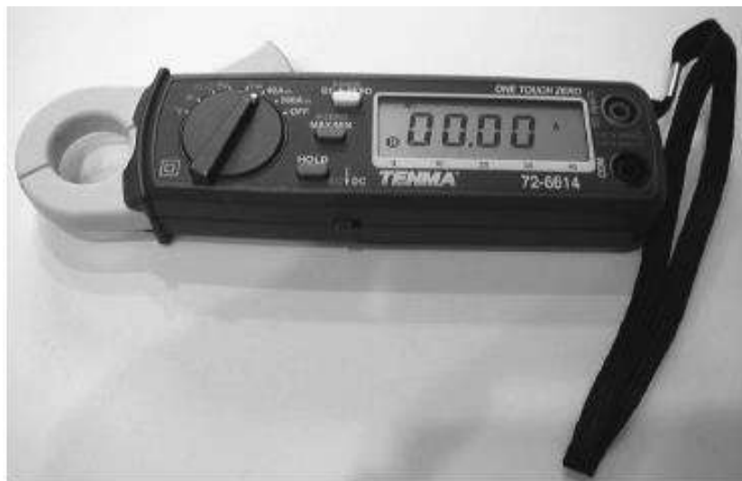
FIGURE: A typical mini clamp-on-type digital multimeter. This meter is capable of measuring alternating current (AC) and direct current (DC) without requiring that the circuit be disconnected to install the meter in series. The jaws are simply placed over the wire and current flow through the circuit is displayed.
