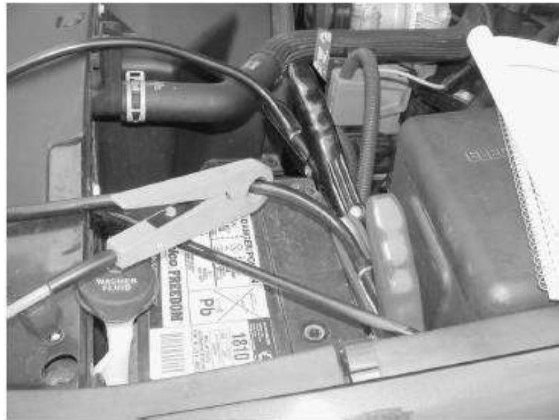
FIGURE: An inductive ammeter clamp is used with all starting and charging testers to measure the current flow through the battery cables.
