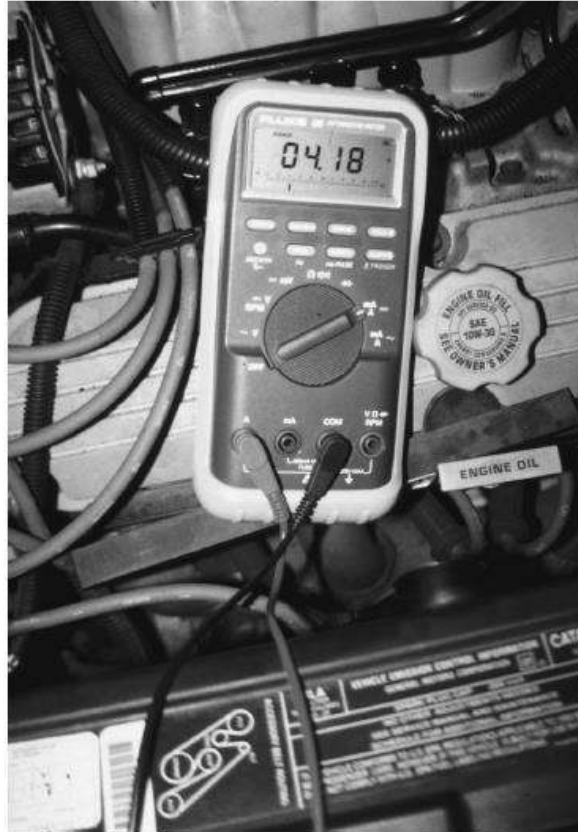
FIGURE: In this digital multimeter set to read DC amperes, note that the red lead is placed in the far left-hand socket of the meter. The meter is displaying the current flow (4.18A) through the electric fuel pump on this General Motors 3800 V6 engine.
