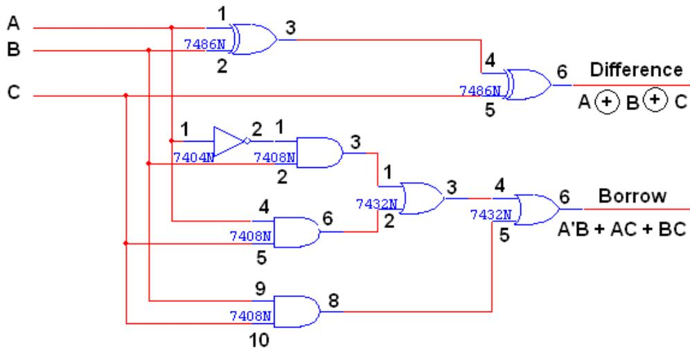
**FULL SUBTRACTOR USING TWO HALF SUBTRACTOR:**
