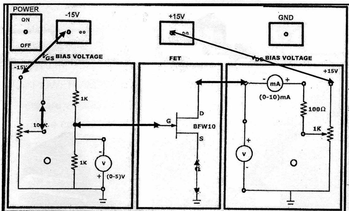
Fig 3.1 WIRING DIAGRAM FET CHARACTERISTICS
