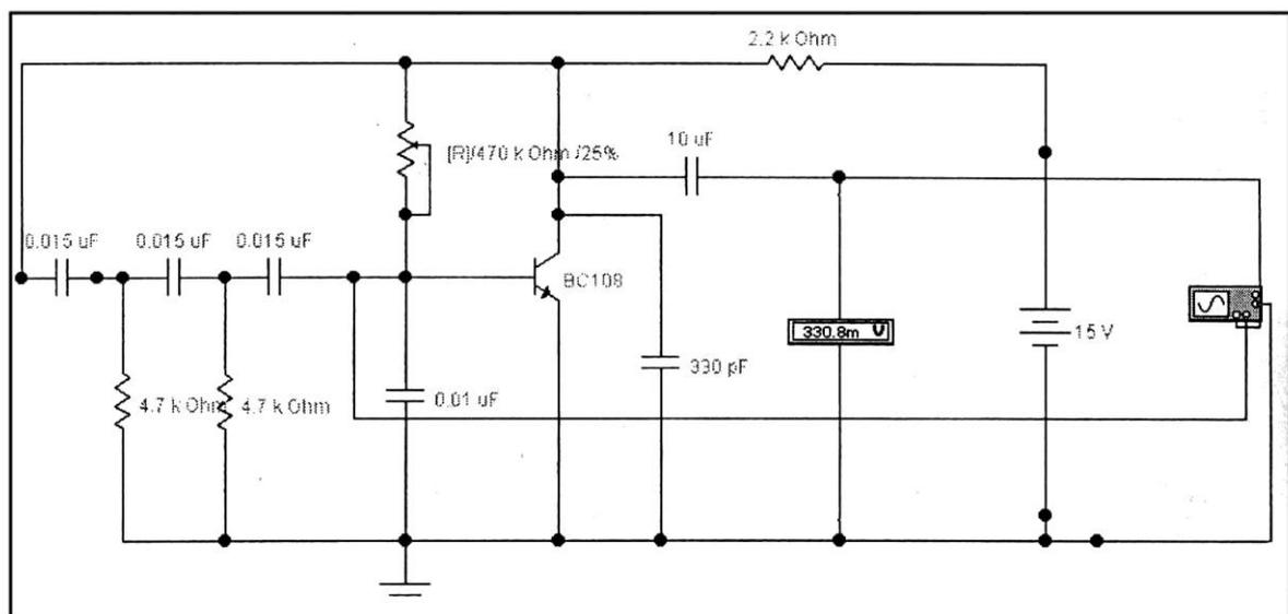
Circuit diagram of RC-Phase Shift Oscillator
