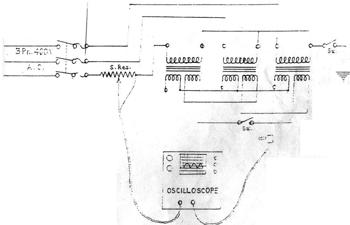
**STUDY OF MAGNETISING CURRENT AND SEC. INDUCED VOLTAGE WAVE SHAPE OF A 3 Phase 3 WINDING TRANSFORMER**
