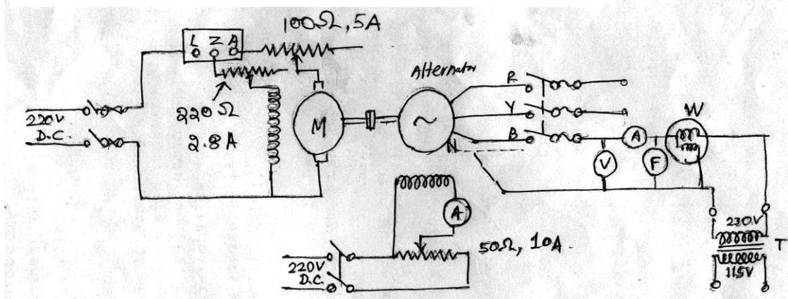
SEPARATION OF IRON LOSS OF A SINGLE PHASE TRANSFORMER
