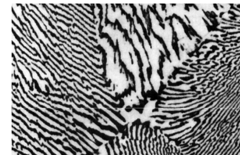
Pb-Sn Eutectic Microstructure
