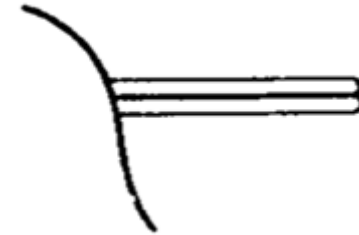
\alpha -Fe plates are now grown new Fe 3 C plates nucleated
