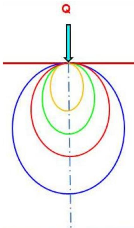
**Fig. 4.1** Isobar diagram (A system of pressure bulbs for a point load- Boussinesq's)
