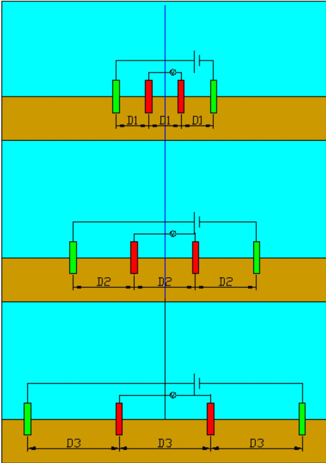
Fig. 25.2. Electrode arrangement for electrical sounding method
