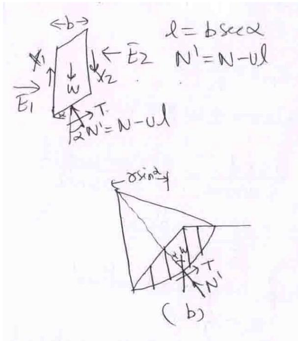
Fig. 13.1 Forces acting on the slices are :
