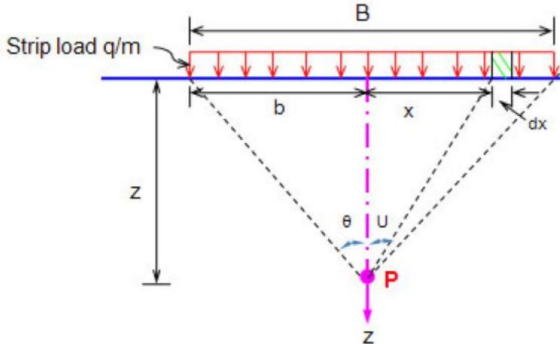
Fig 5.1 Vertical stress due to strip load point 'P' below the centre
