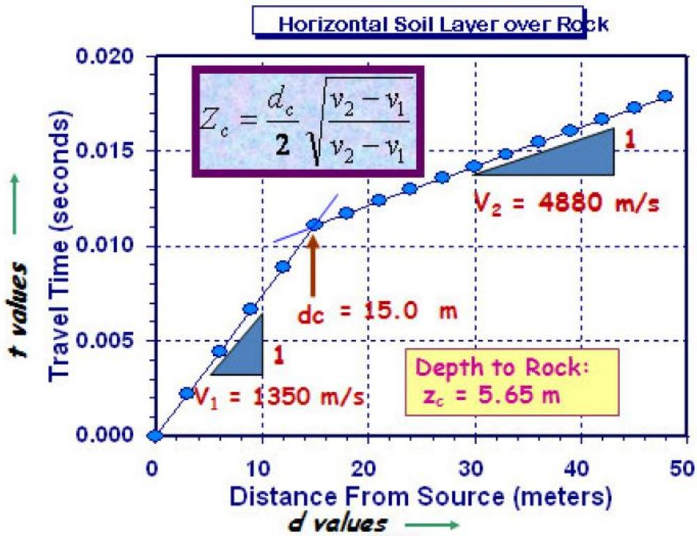
**Fig.24.4 Plot of Travel time versus distance obtained from seismic refraction method**
