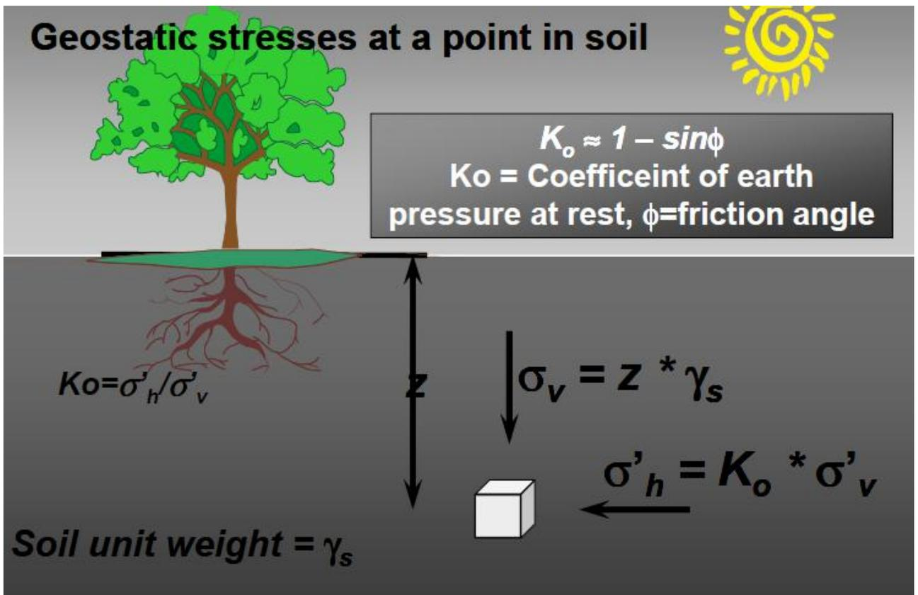
Fig. 1.3 Geostatic stresses at a point in soil
