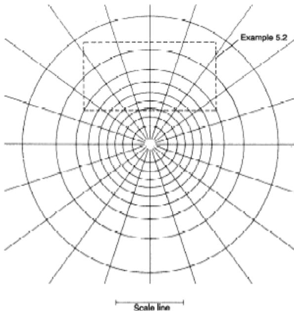
Fig 6.2 *vertical stress increase at z*
