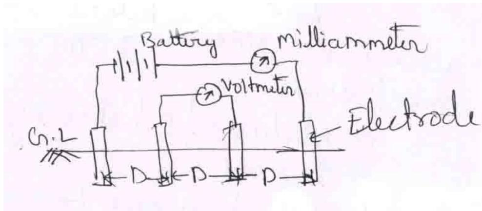
Fig. 15.3 Wenner configuration for electrical resistivity.
