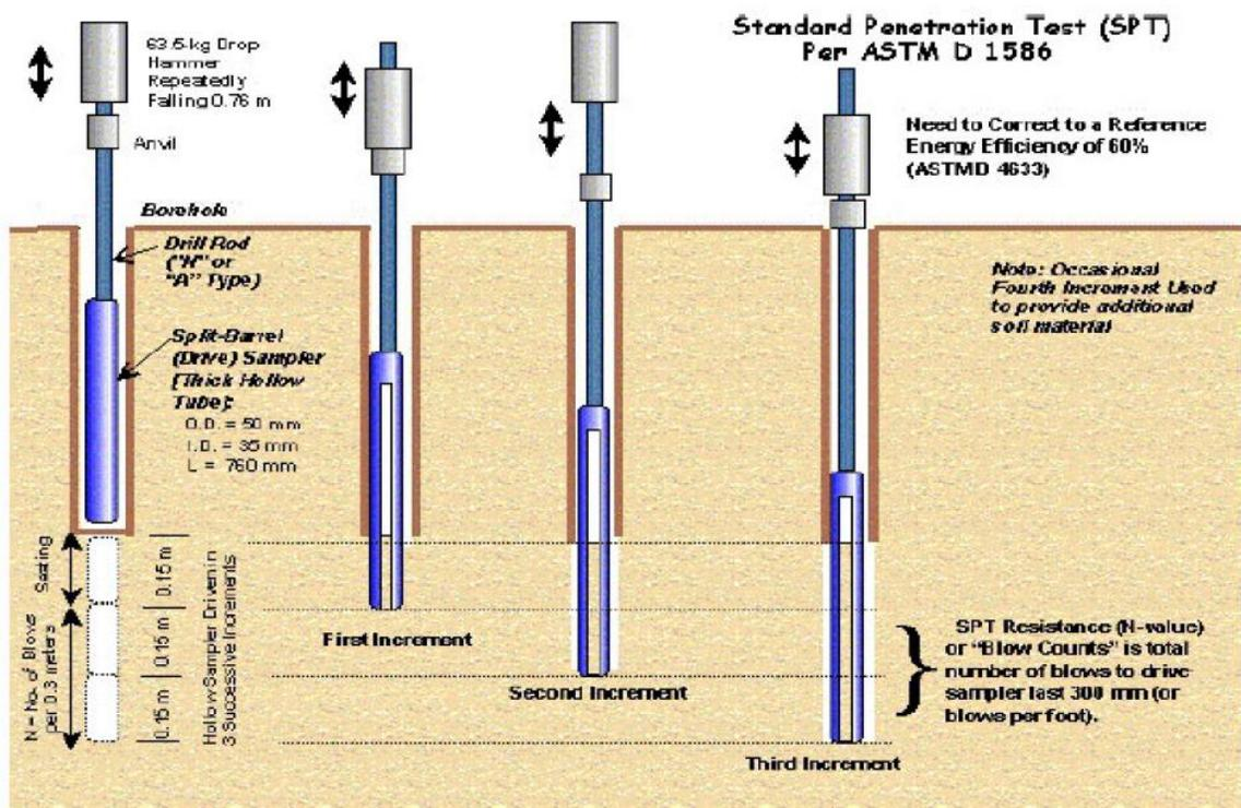
Fig.21.2 Stages of Standard Penetration testing
