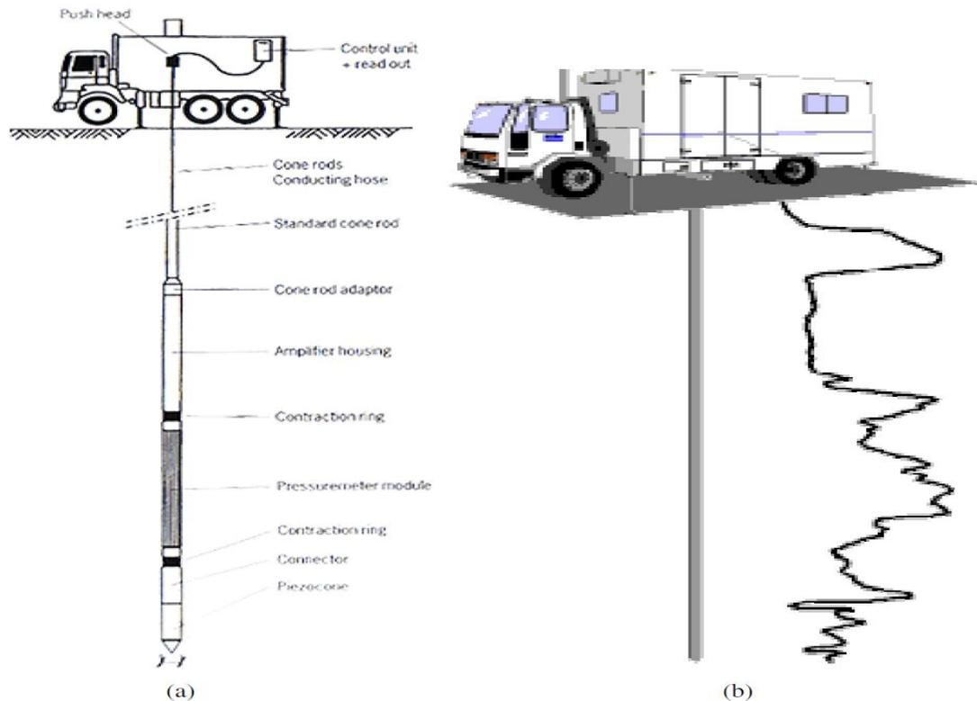
**Fig.22.1 Cone penetration set up**
