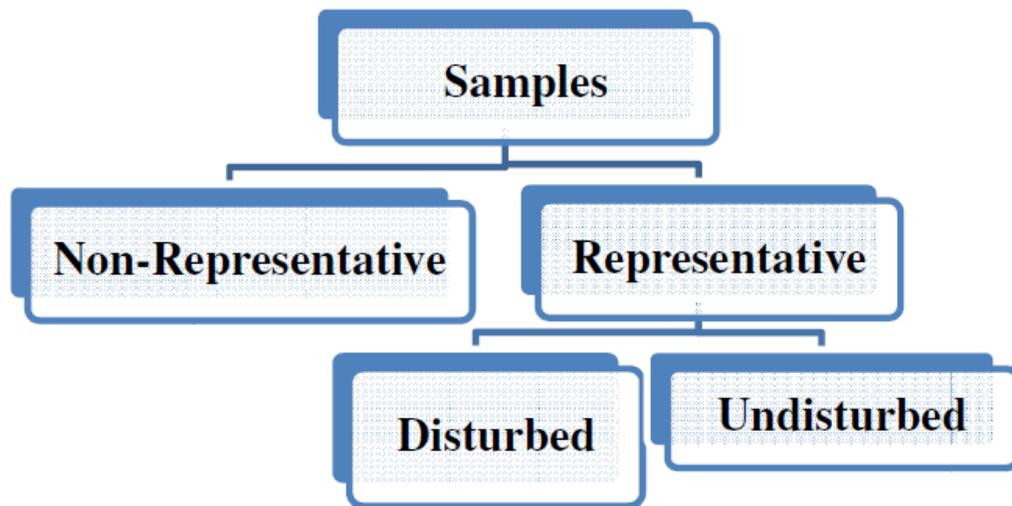
**Fig. 18.2 Types of soil samples**
