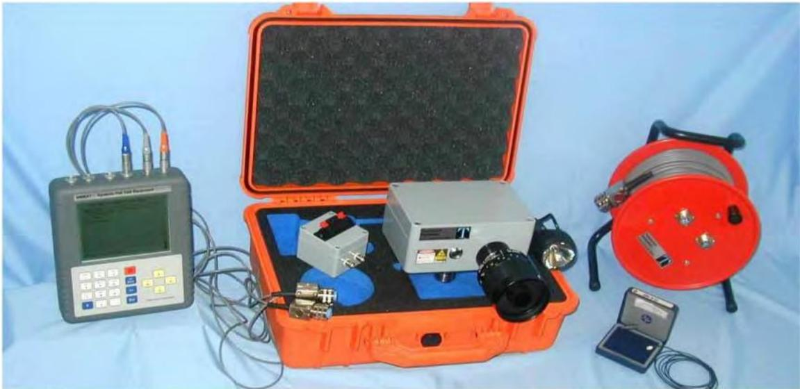
**Figure 40.2:** Complete SIMBAT kit including data collection unit, accelerometers, digital theodolite cable reels and waterproof carry case
