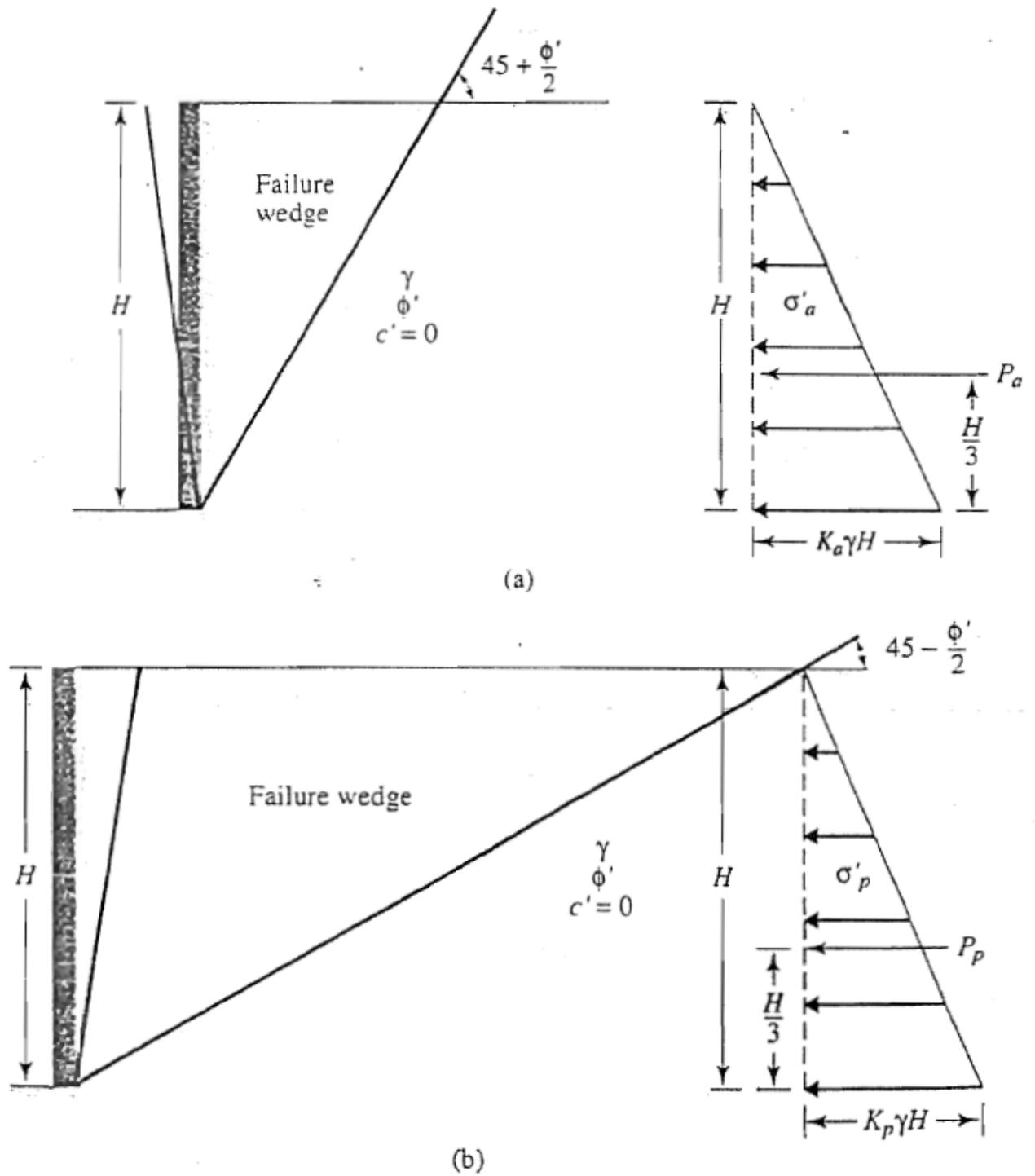
Fig. 8.3 Pressure distribution against a retaining wall for cohesionless soil backfill with horizontal ground surface (a) Rankine's active state (b) Rankine's passive state
