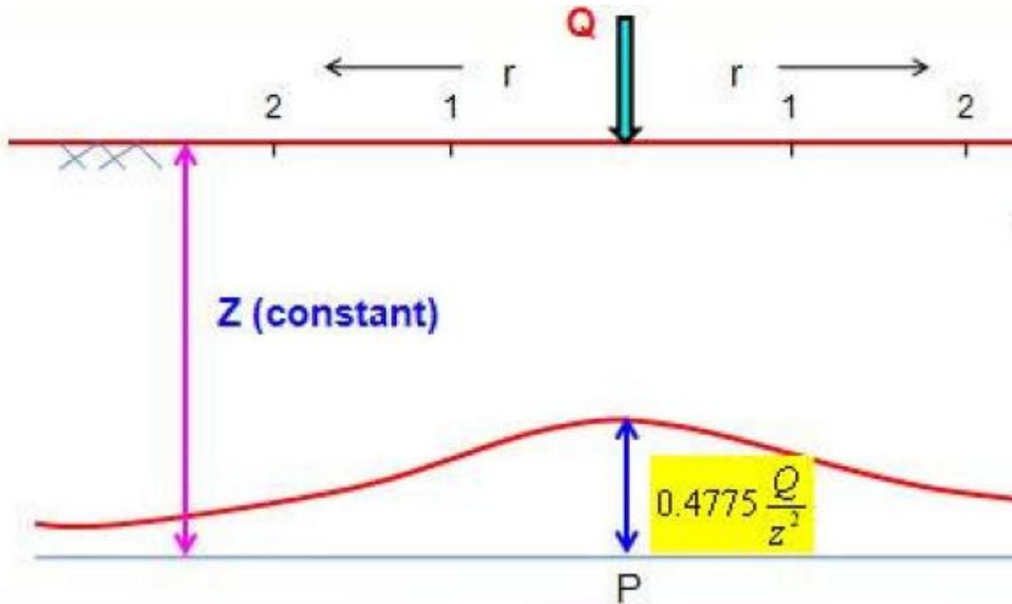
**Fig. 3.2** Vertical stress distribution on a horizontal plane at depth 'z' ( Boussinesq's)
