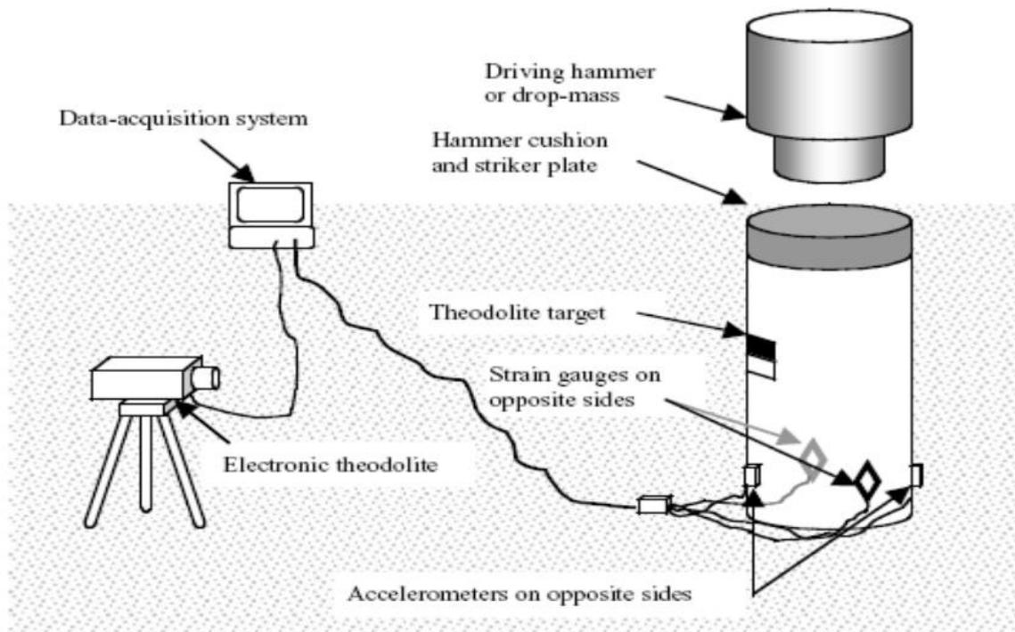
**Figure 40.1:** Schematic of SIMBAT Instrumentation
