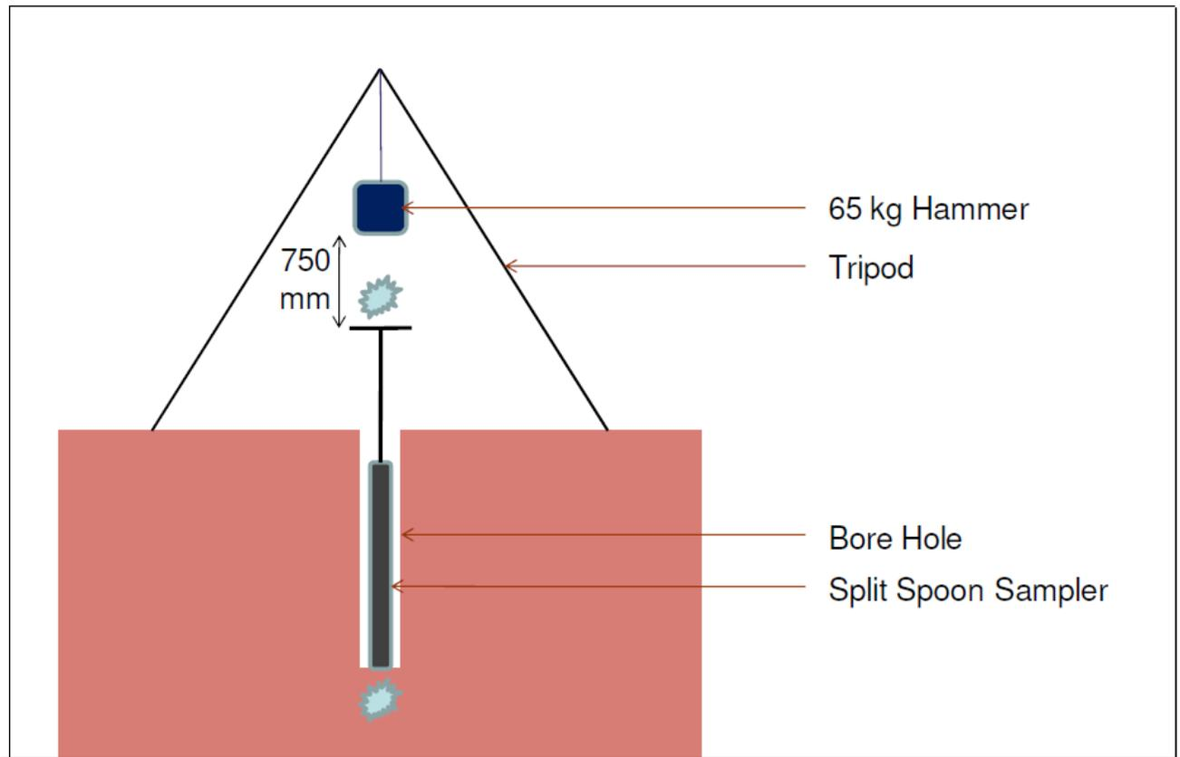
Fig. 14.1 Typical set up for Standard Penetration test assembly
