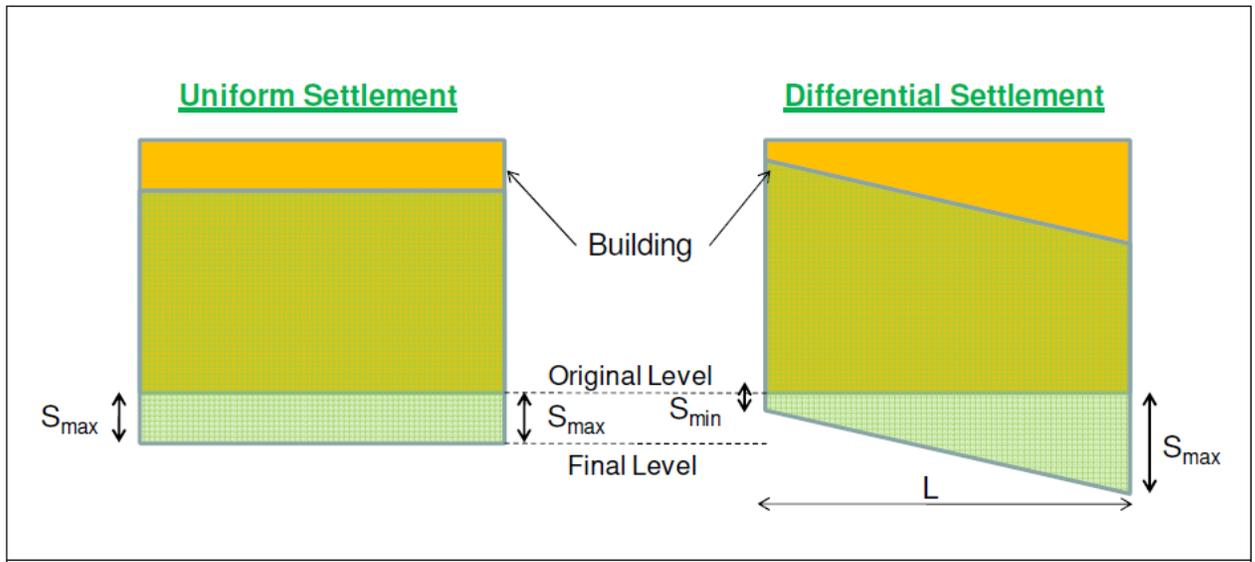
Fig. 29.1 : Concepts of uniform and differential settlement
