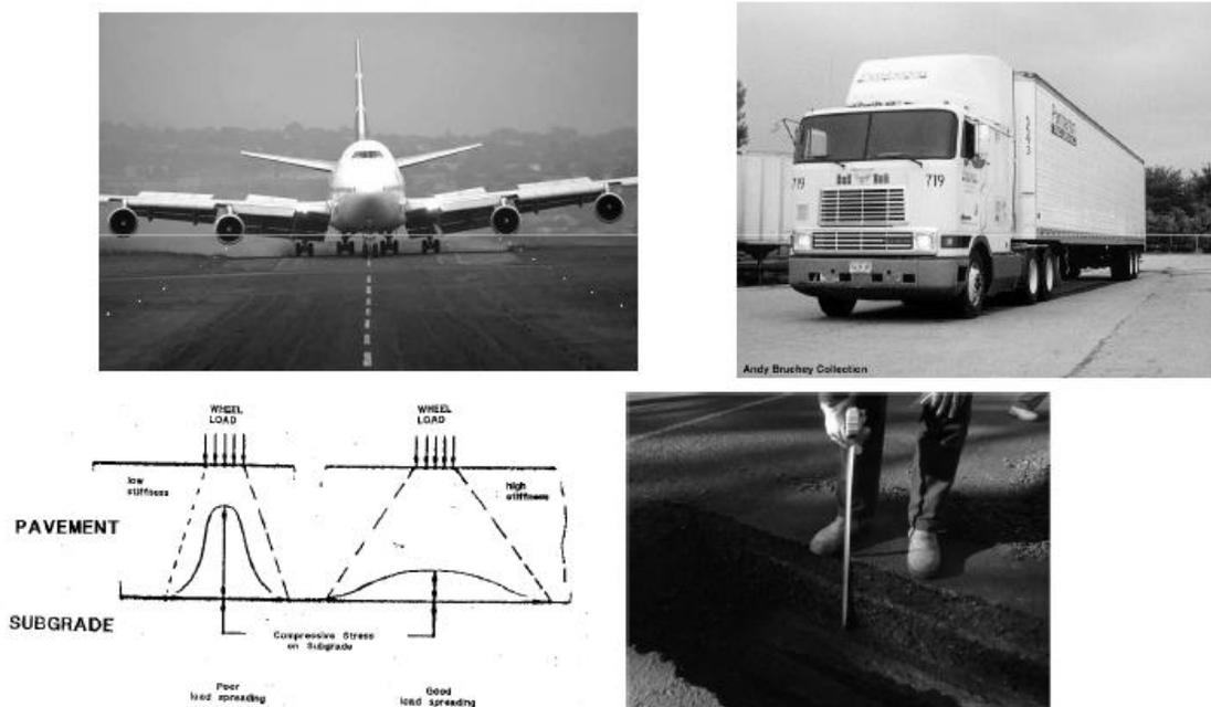
Fig. 1.4 Subsurface stresses in road pavements and airport runways are increased by wheel load on the surface
