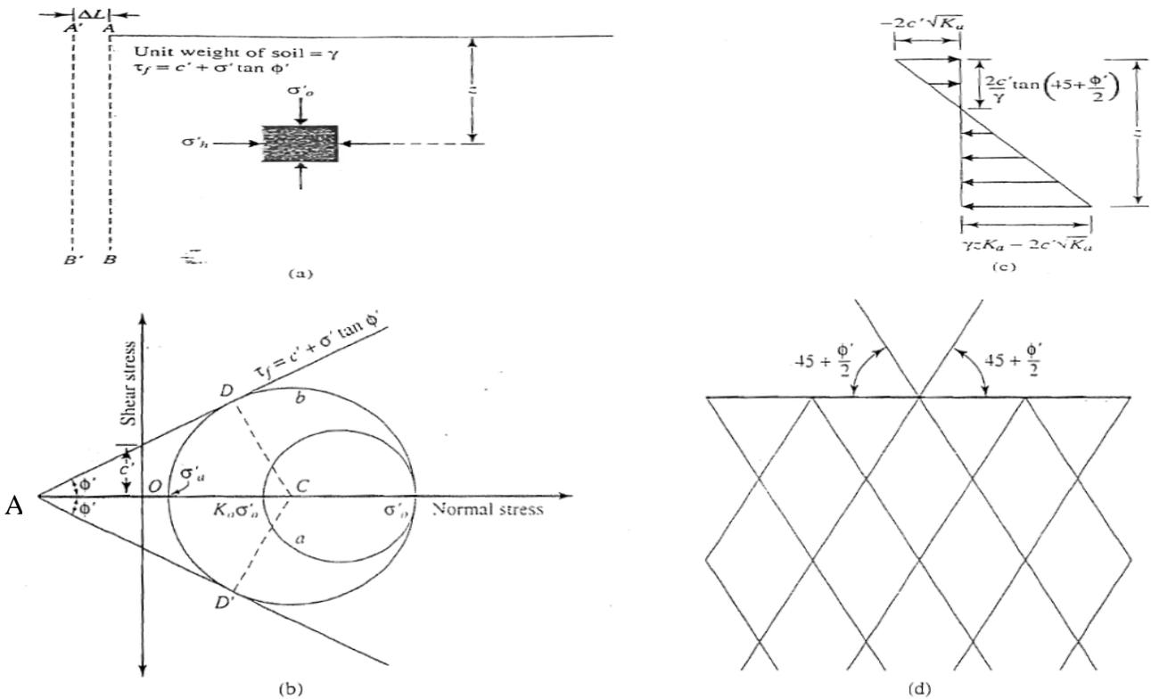
Fig. 8.1 Rankine's active earth pressure
