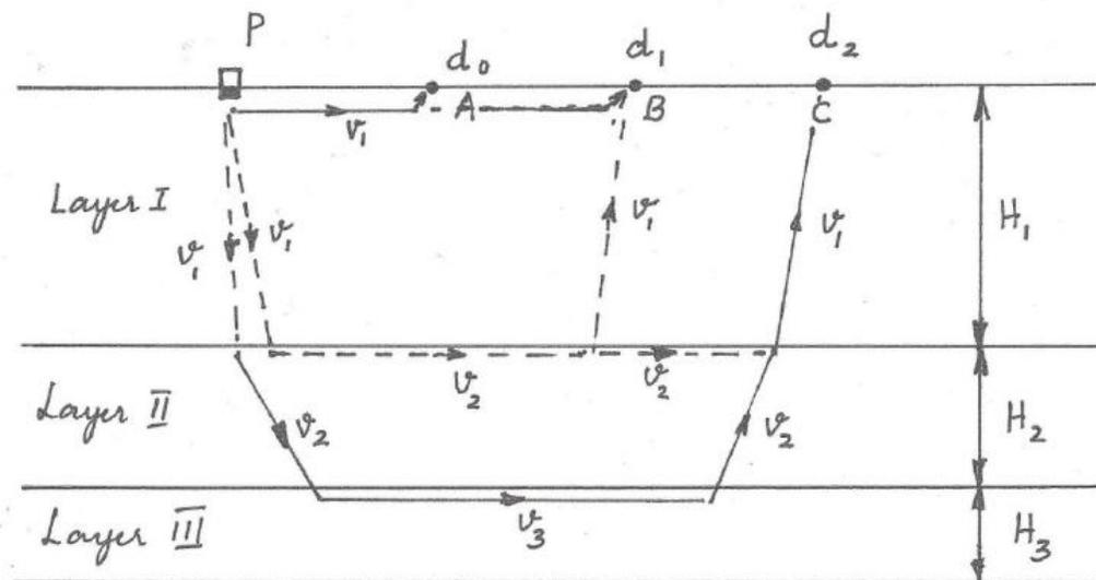
Fig. 24.3 Seismic refraction method
