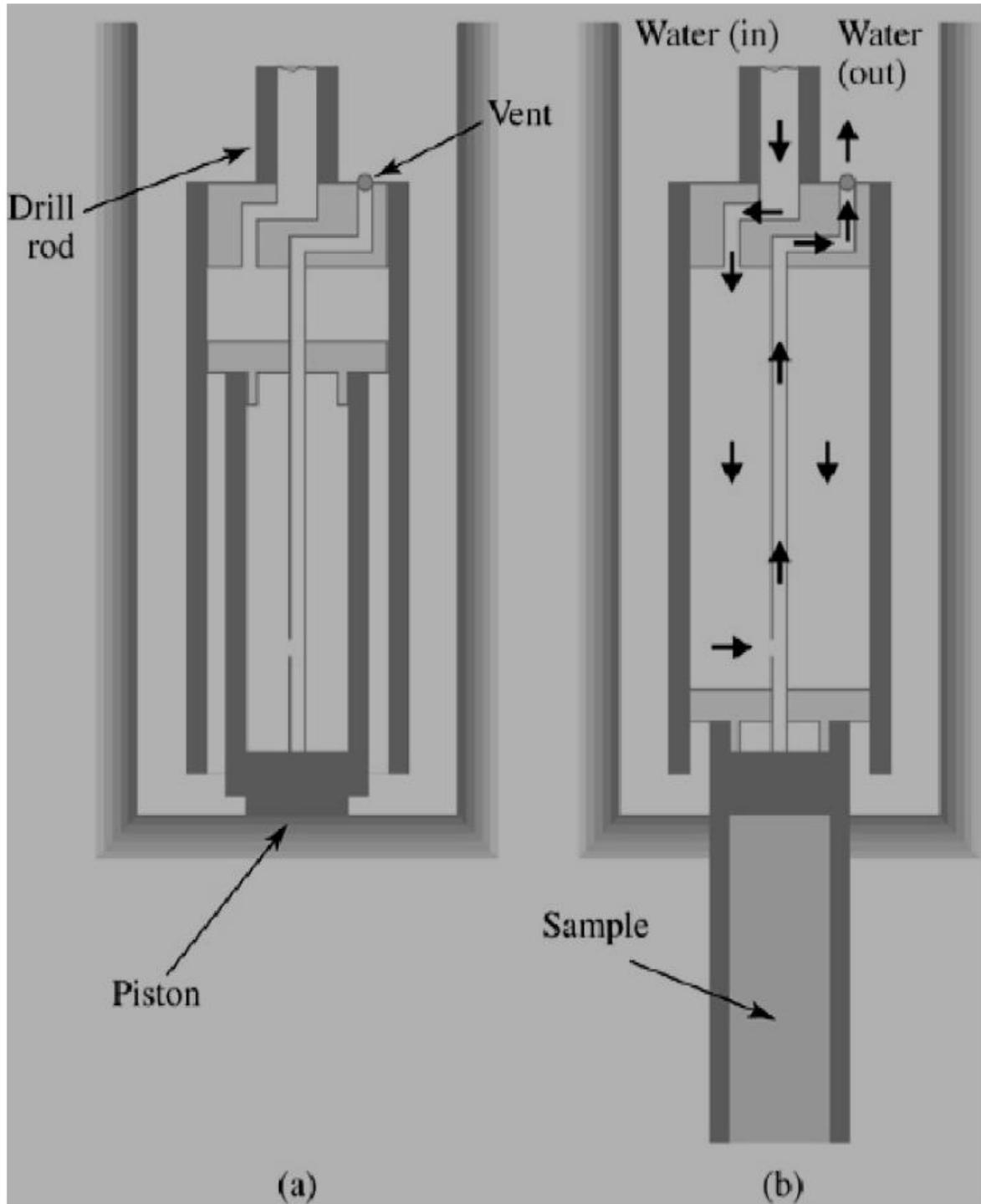
**Fig.20.1** Piston sampler
