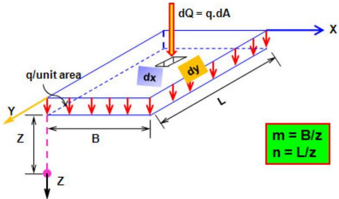
Fig 6.1 Vertical stress of a uniformly loaded rectangular area
