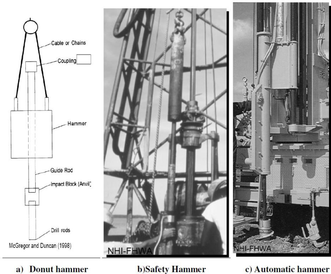
**Fig. 21.3 Types of SPT hammers**
