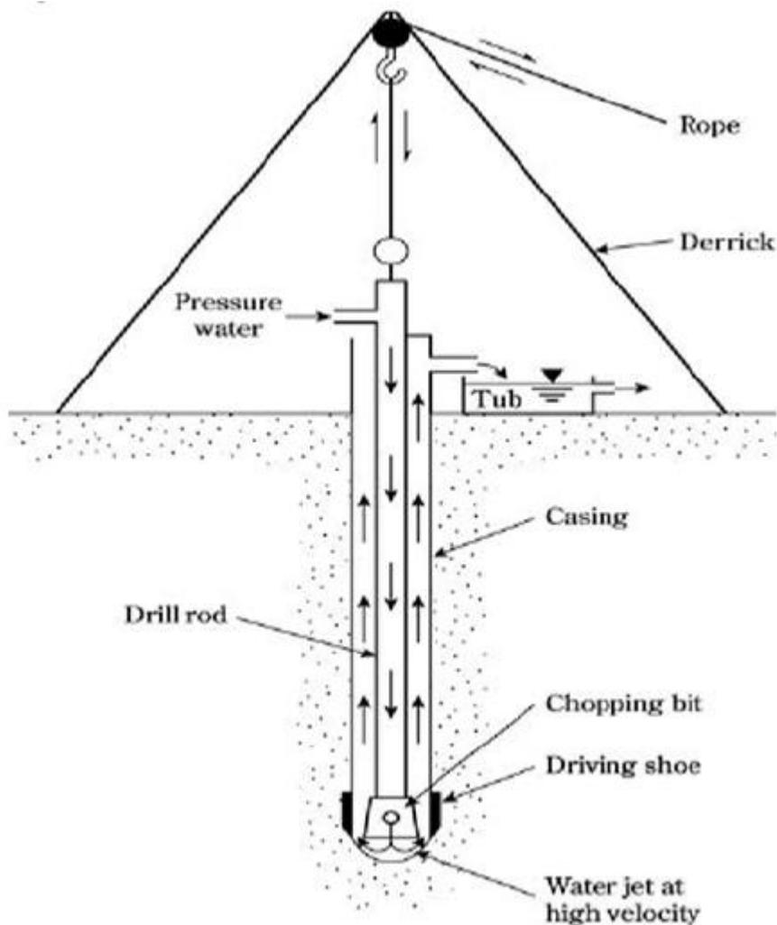
**Fig.18. 1 Wash Boring set up**
