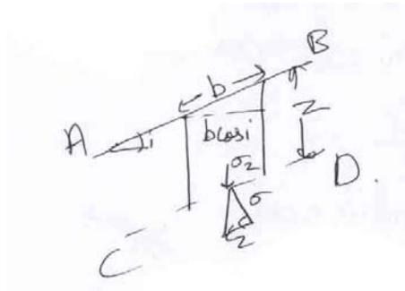
Fig. 11.2 Infinite slope
