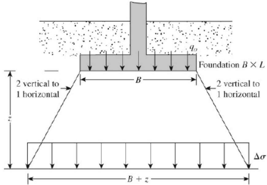
Fig 6.4 Two is to one method
