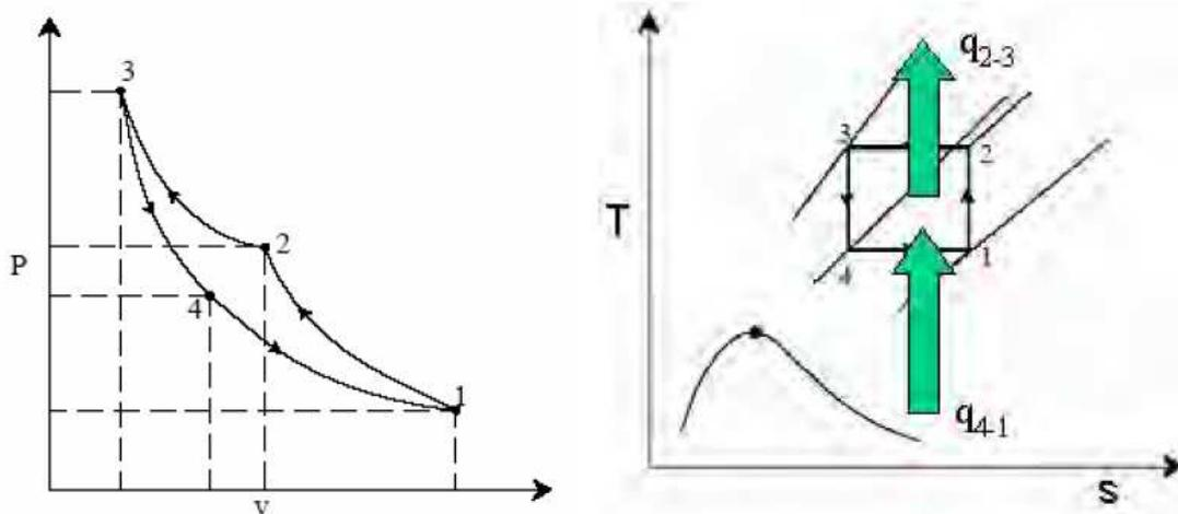
**Fig. 1(b).** Reverse Carnot refrigeration system in  $P$ - $v$  and  $T$ - $s$  coordinates
