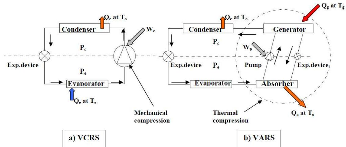
*Figs.14.2: a) Vapour compression refrigeration system (VCRS)
