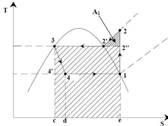
**Fig.10.6(b).** Comparative evaluation of heat rejection rate of VCRS and Carnot cycle
