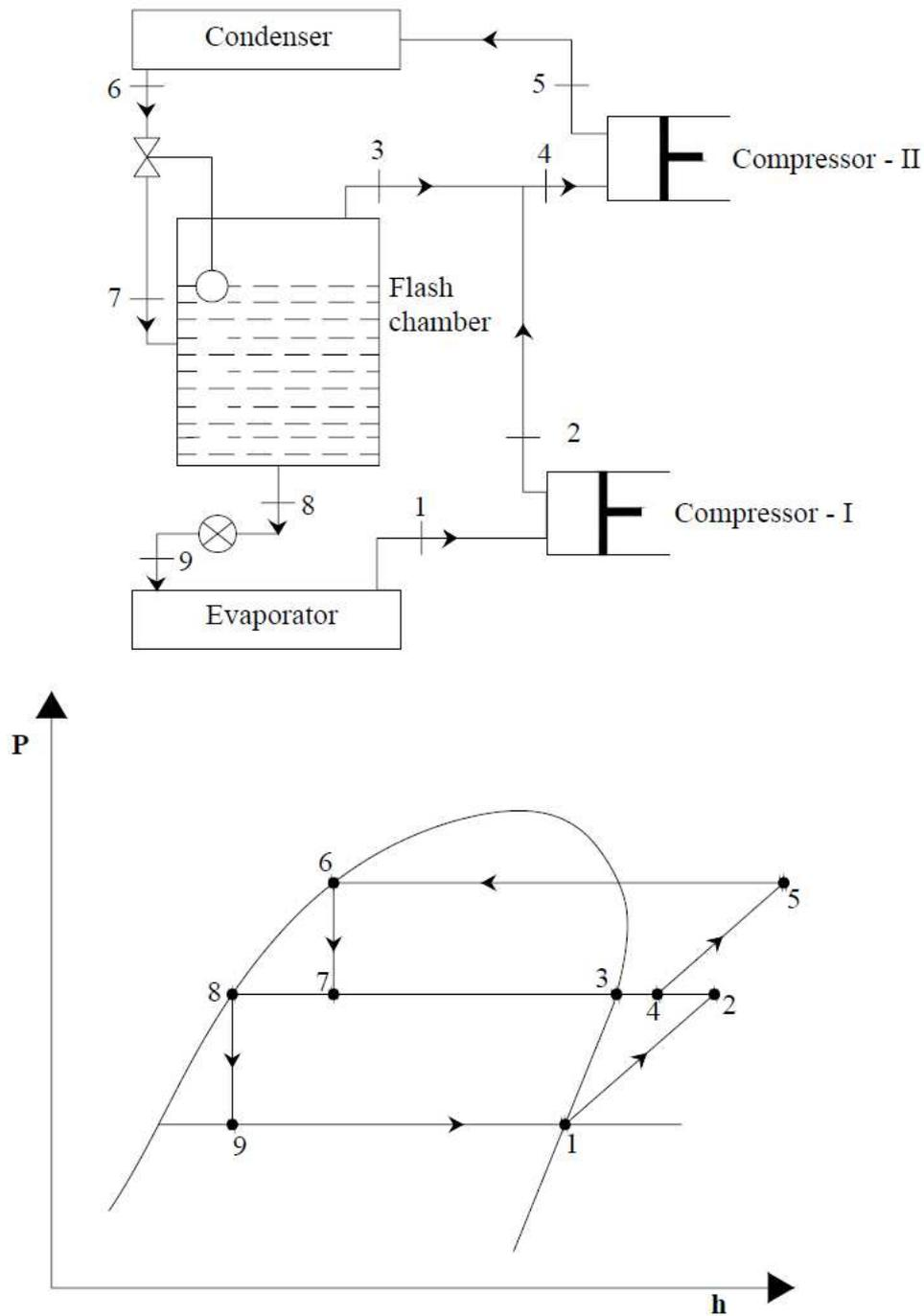
*Fig.12.8: A two-stage compression system with flash tank for flash gas removal only
