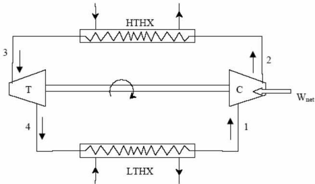
**Fig. 2(a).** Schematic of a closed reverse Brayton cycle
