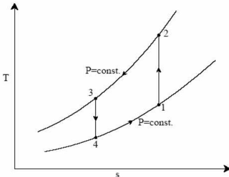
**Fig. 2(b).** Reverse Brayton cycle in T-s plane
