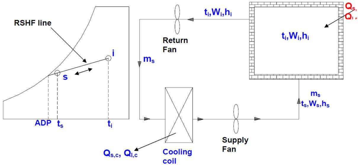
**Fig.30.1:** A simple, 100% re-circulation type air conditioning system
