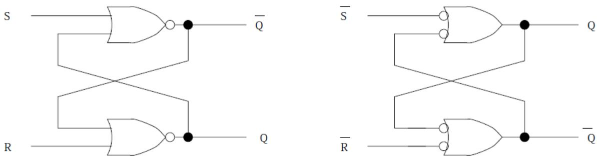
Figure 1 : Two equivalent versions of an SR flip-flop (or “SR latch”).
