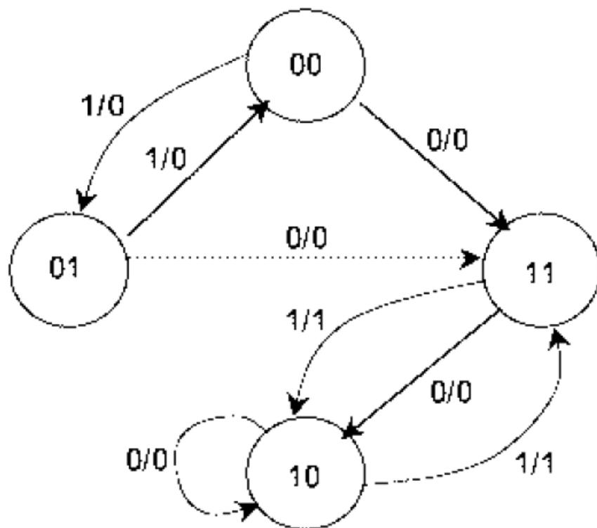
Figure 5. State Diagram of circuit in Figure 4.
