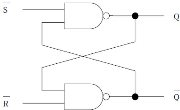
Figure 2 : Yet another equivalent SR flip-flop.
