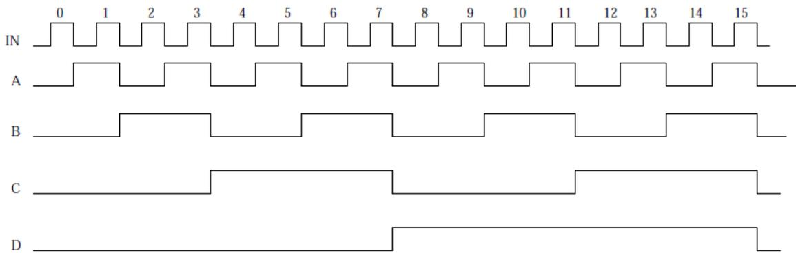
Figure 2 : Waveforms generated by the ripple counter.
