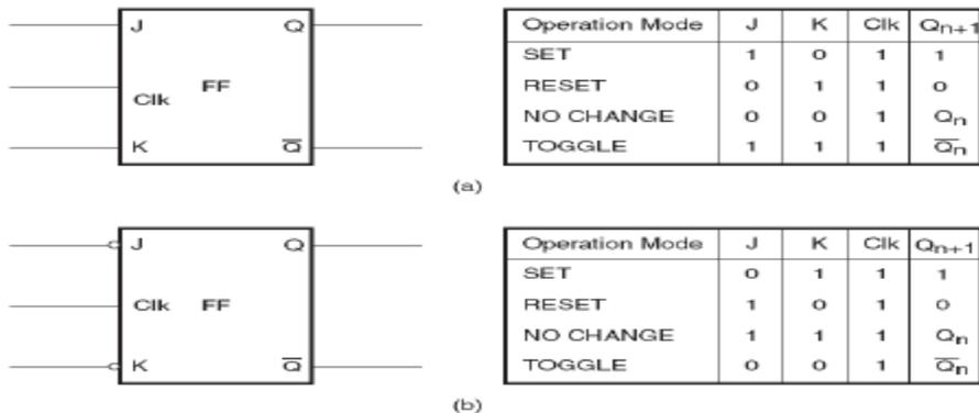
FIG a. JK flip flop with active high inputs, b. JK flip flop with active low inputs
