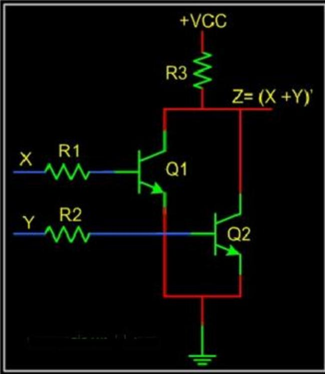
A basic circuit of an RTL NOR gate consists of two transistors Q1 and Q2, connected as the figure above. When either input X or Y is driven HIGH, the corresponding transistor goes to saturation and output Z is pulled to LOW.
