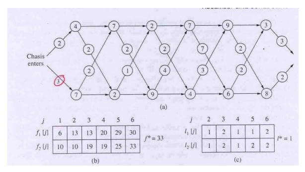
Illustration of assembly line scheduling procedure.
