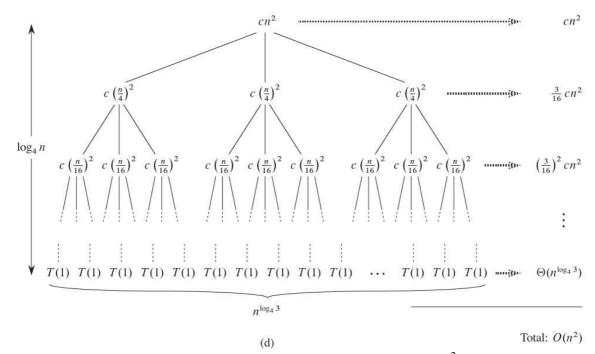
Constructing a recursion tree for the recurrence T (n)= 3T (n=4) + cn<sup>2</sup>.. Part (a) shows T (n), which progressively expands in (b)–(d) to form the recursion tree. The fully expanded tree in part (d) has height  $\log_4 n$  (it has  $\log_4 n + 1$  levels).
