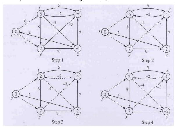
Stepwise working procedure of Bellman Ford Algorithm
