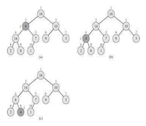
**Figure:** The action of MAX-HEAPIFY (A, 2), where heap-size = 10. (a) The initial configuration, with A [2] at node i = 2 violating the max-heap property since it is not larger than both children. The max-heap property is restored for node 2 in (b) by exchanging A [2] with A[4], which destroys the max-heap property for node 4. The recursive call MAX-HEAPIFY (A,4)
