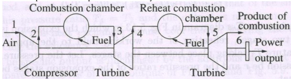
**Fig. 46. Arrangement of reheat cycle**
