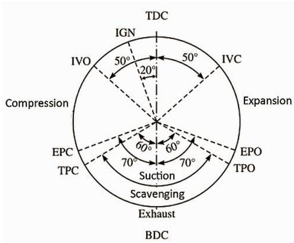
**Fig. 6. Port timing diagram for 2-stroke engine**
