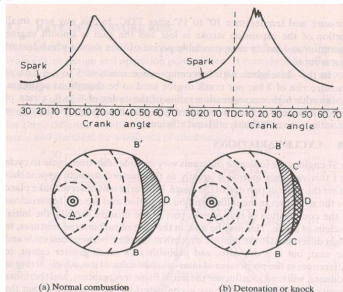
**Fig. 26. Detonation in SI engine**
