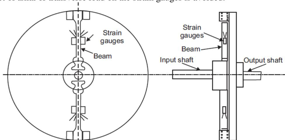
Fig. 33. Transmission dynamometer
