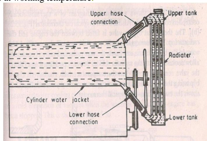
**Fig. 37. Thermo-syphon cooling**
