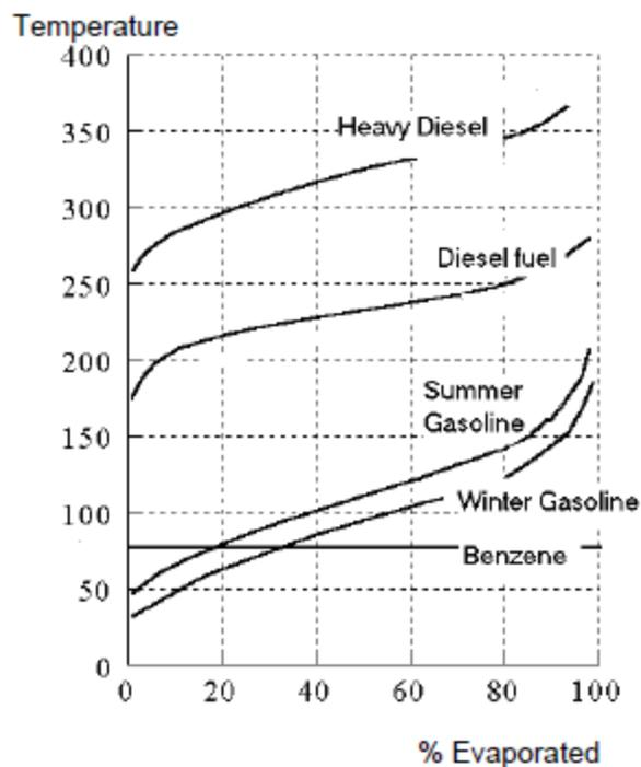
**Fig. 12. Distillation curve**
