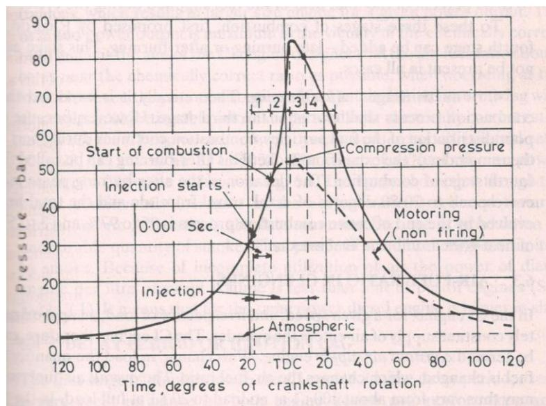
**Fig. 27. Stages of combustion in CI engine**
