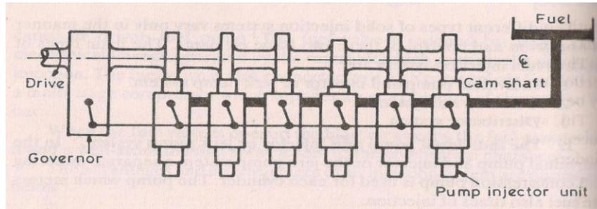
**Fig. 19. Unit injector**
