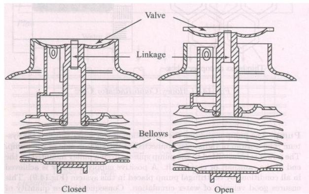
**Fig. 38. Bellows type thermostat**
