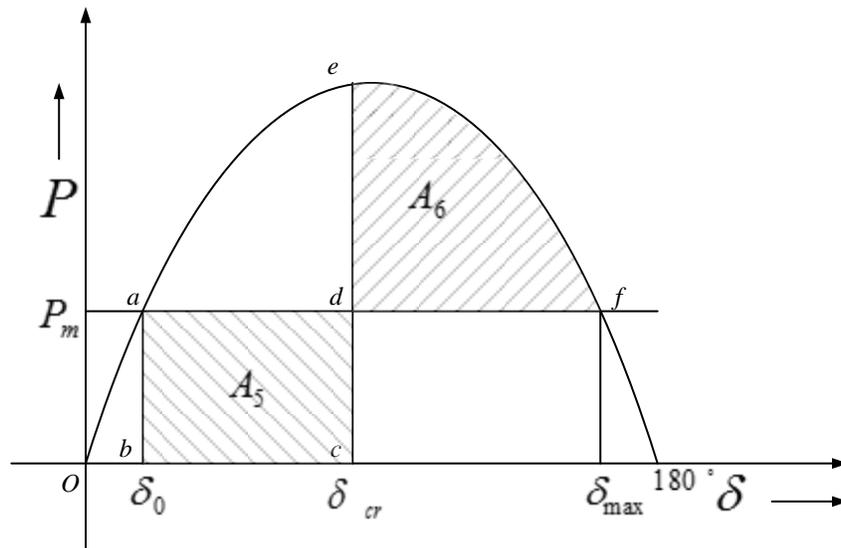
FIG.-4.4 POWER ANGLE CURVE FOR THE GENERATOR (CRITICAL CASE)
