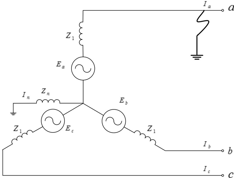
FIG.-6.4 SINGLE LINE TO GROUND FAULT AT TERMINAL *phase-'a'* OF THE UNLOADED GENERATOR
