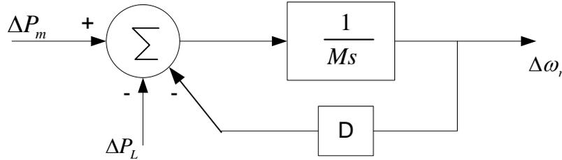
FIG.-7.4 BLOCK DIAGRAM OF GENERATOR WITH LOAD DAMPING
