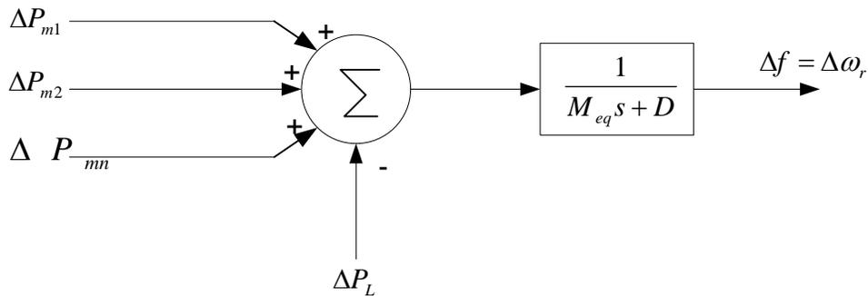
FIG.-7.14 EQUIVALENT SYSTEM GENERATORS AND LOAD
