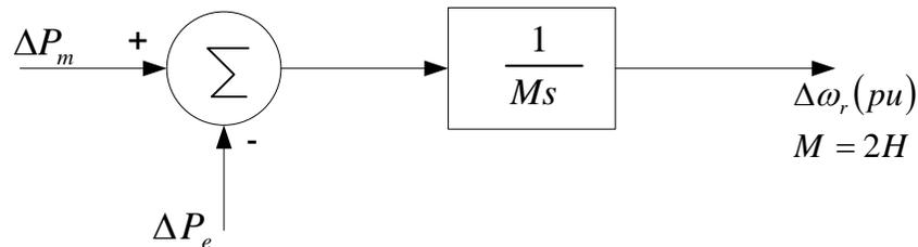
FIG.-7.3 BLOCK DIAGRAM OF GENERATOR
