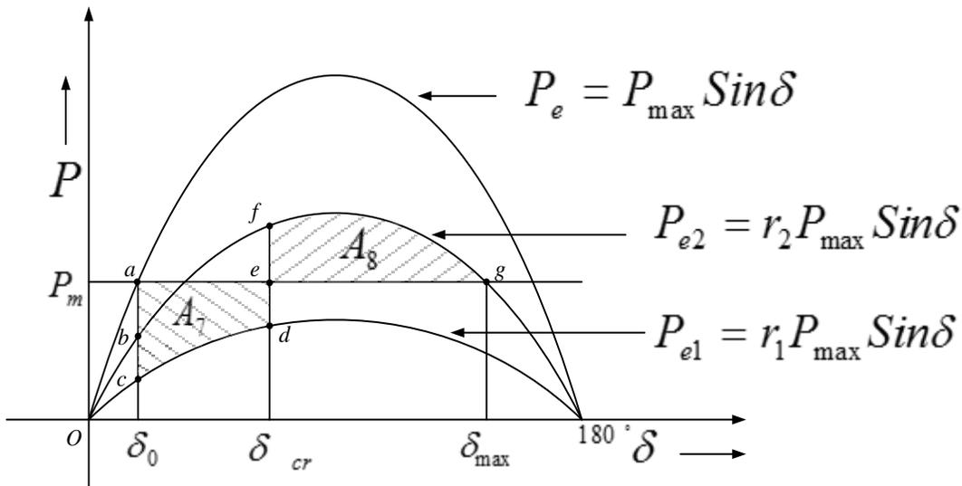
FIG.-4.5 POWER ANGLE CURVE FOR THE GENERATOR (POWER TRANSMITTED DURING FAULT)
