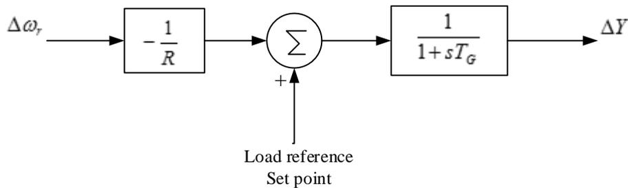
FIG.-7.12 BLOCK DIAGRAM OF GOVERNOR WITH LOAD REFERENCE CONTROL
