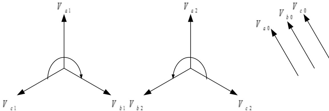
FIG.-6.1 SYMMETRICAL COMPONENTS OF THREE PHASE SYSTEM
