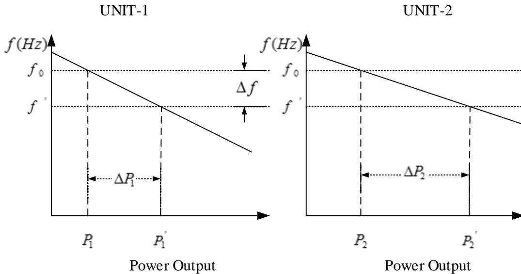
FIG.-7.11 LOAD SHARING BETWEEN TWO GENERATORS HAVING DIFFERENT REGULATION
