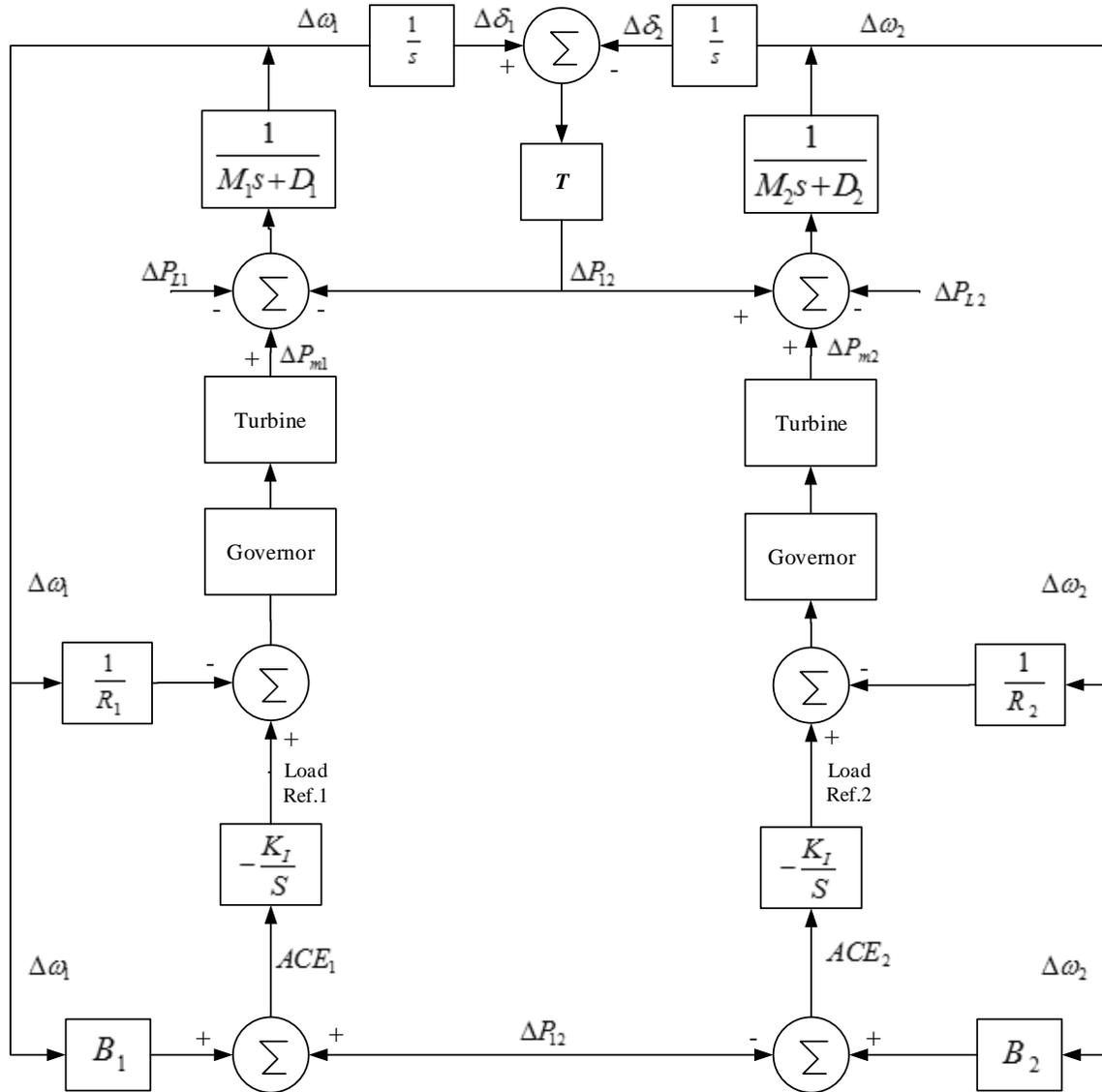
FIG.-7.18 BLOCK DIAGRAM FOR CONTROL OF TWO INTERCONNECTED POWER SYSTEM WITH SUPPLEMENTARY CONTROL
