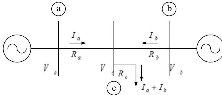
FIG.-5.1 POWER SYSTEM HAVING TWO GENERATING STATION AND A LOAD
