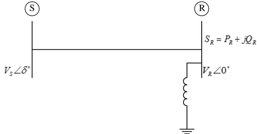
FIG.-1.3 TRANSMISSION LINE WITH SHUNT COMPENSATION
