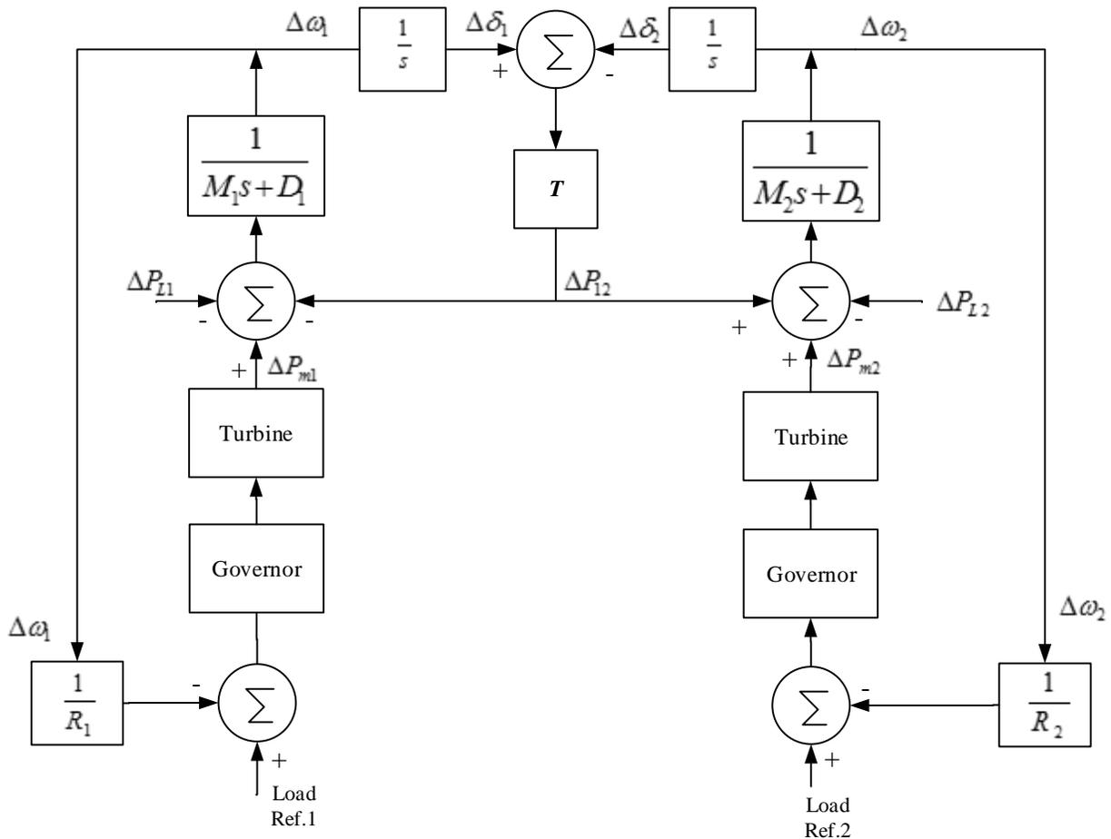
FIG.-7.17 BLOCK DIAGRAM FOR CONTROL OF TWO INTERCONNECTED POWER SYSTEM FOR PRIMARY SPEED CONTROL
