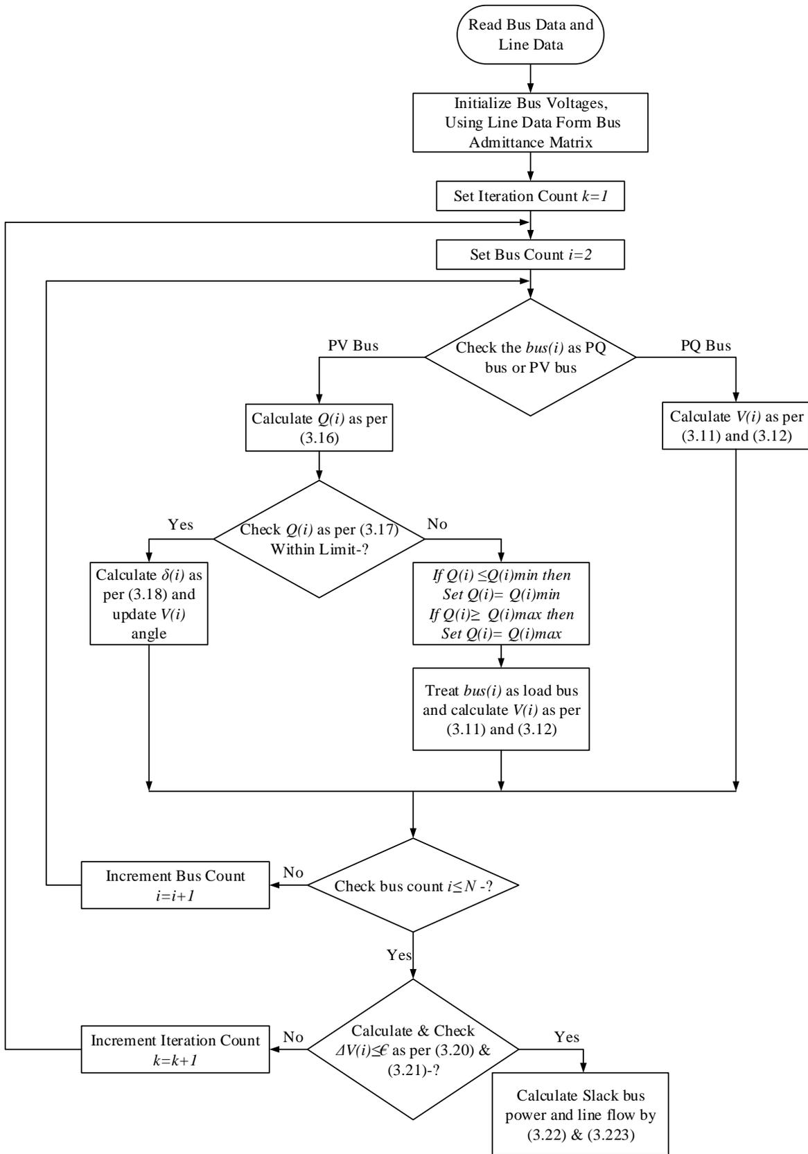
FIG.-3.4 FLOW CHART FOR LOAD FLOW USING GAUSS SEIDEL METHOD
