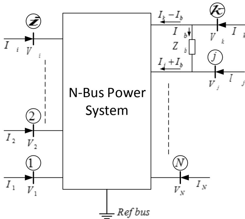
FIG.-2.5 ADDITION OF NEW LINK BETWEEN TWO EXISTING BUSES
