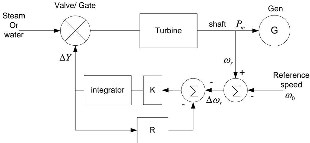
FIG.-7.7 BLOCK DIAGRAM OF GOVERNOR WITH STEADY STATE FEEDBACK:
