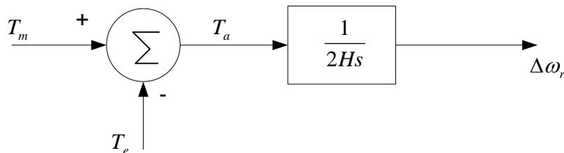
FIG.-7.2 BLOCK DIAGRAM OF GENERATOR
