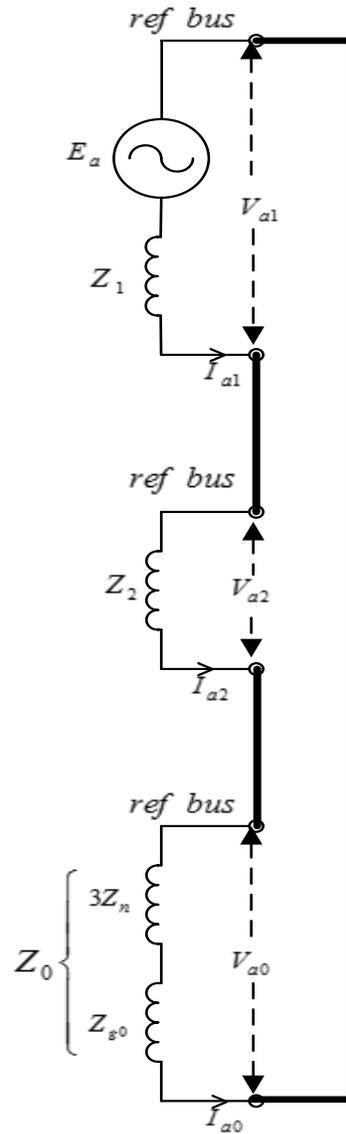
FIG.-6.5 EQUIVALENT NETWORK FOR UNLOADED GENERATOR HAVING SINGLE LINE TO GROUND FAULT
