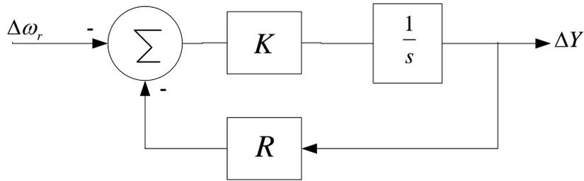
FIG.-7.8 SIMPLIFIED BLOCK DIAGRAM OF GOVERNOR WITH STEADY STATE FEEDBACK:
