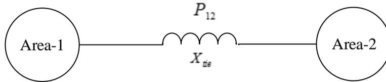
FIG.-7.17 ELECTRICAL EQUIVALENT OF TWO INTERCONNECTED POWER SYSTEM
