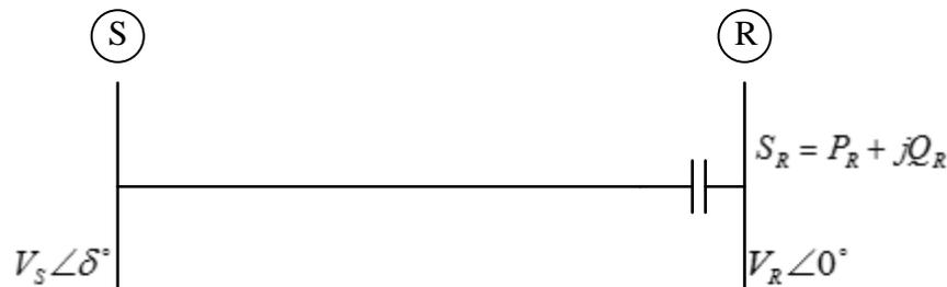
FIG.-1.2 TRANSMISSION LINE WITH SERIES COMPENSATION
