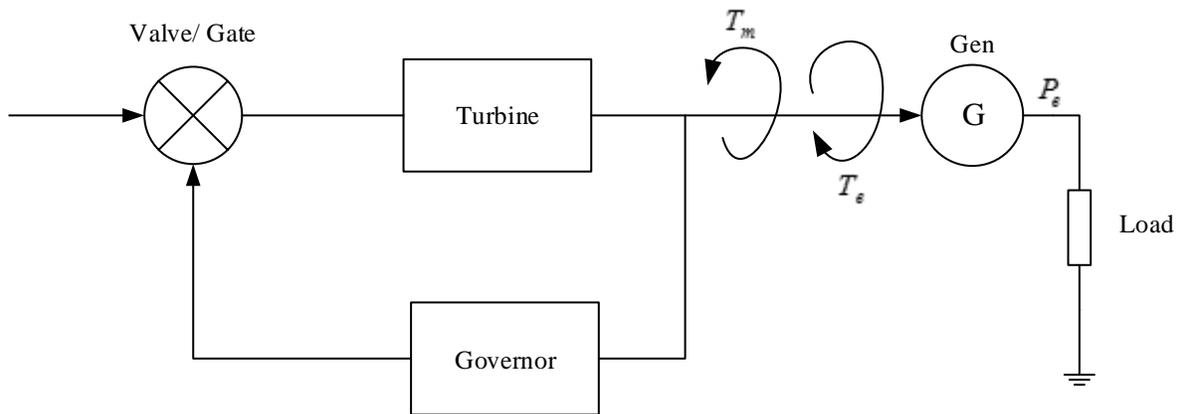
FIG.-7.1 SCHEMATIC BLOCK DIAGRAM OF ACTIVE POWER CONTROL WITH FEEDBACK
