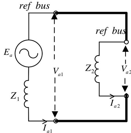
FIG.-6.7 EQUIVALENT NETWORK FOR UNLOADED GENERATOR HAVING LINE TO LINE FAULT
