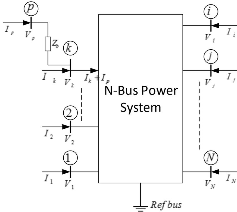
FIG. 2.3 ADDITION OF NEW BUS 'p' TO AN EXISTING BUS 'k'
