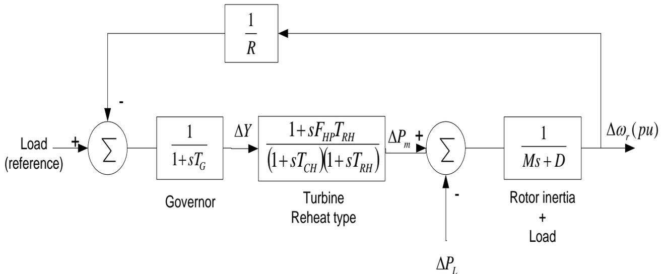
FIG.-7.15 COMPLETE BLOCK DIAGRAM OF GENERATOR WITH TURBINE GOVERNING SYSTEM
