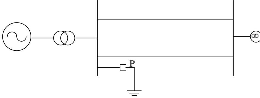
FIG.-4.1 SINGLE MACHINE INFINITE BUS SYSTEM
