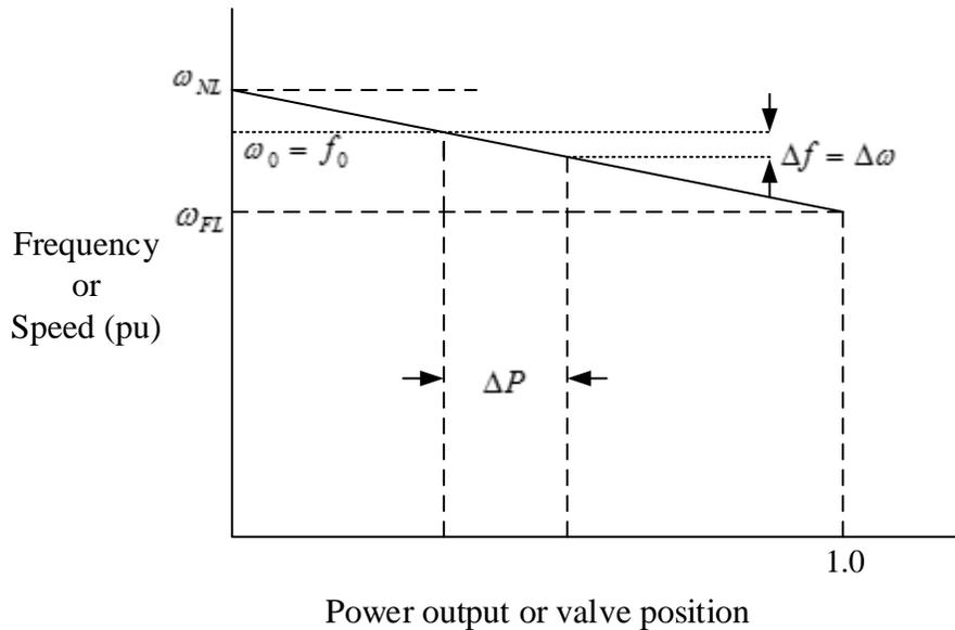
FIG.-7.10 IDEAL STEADY STATE CHARACTERISTICS OF GOVERNOR WITH SPEED DROOP
