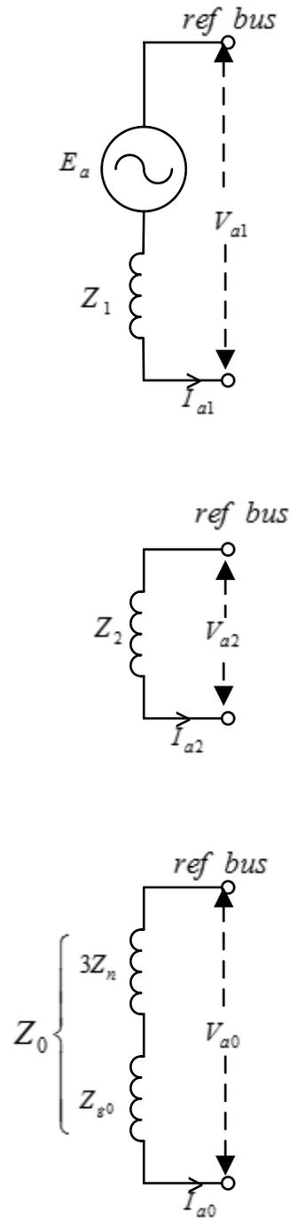
FIG.-6.3 VOLTAGE OF *phase-'a'* OF UNLOADED GENERATOR
