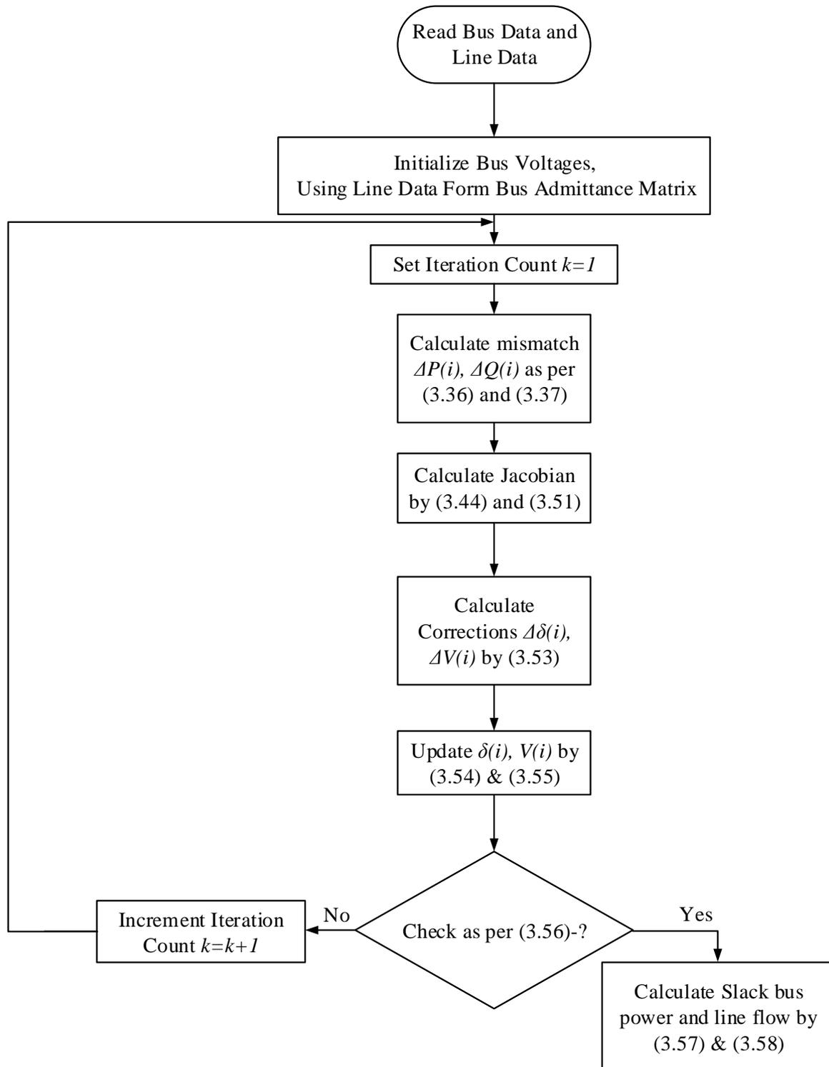
FIG.-3.4 FLOW CHART FOR LOAD FLOW USING NEWTON-RAPHSON METHOD
