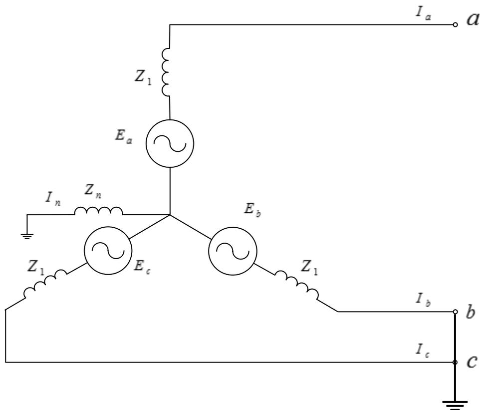
FIG.-6.8 DOUBLE LINE TO GROUND FAULT INVOLVING TERMINALS *phase-'b'* AND *phase-'c'* OF THE UNLOADED GENERATOR
