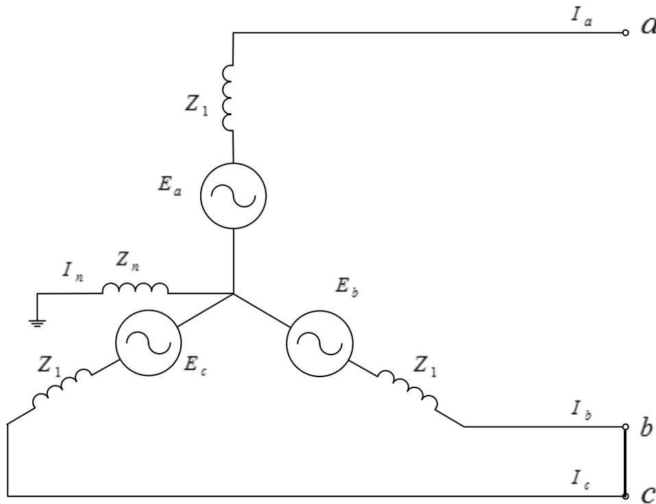
FIG.-6.6 LINE TO LINE FAULT INVOLVING TERMINALS *phase-'b'* AND *phase-'c'* OF THE UNLOADED GENERATOR
