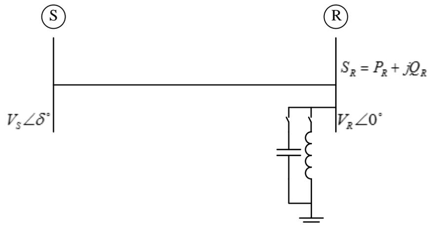
FIG.-1.4 TRANSMISSION LINE WITH SHUNT COMPENSATION
