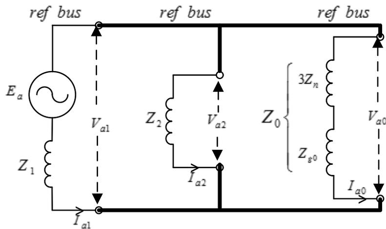
FIG.-6.9 EQUIVALENT NETWORK FOR UNLOADED GENERATOR HAVING DOUBLE LINE TO GROUND FAULT
