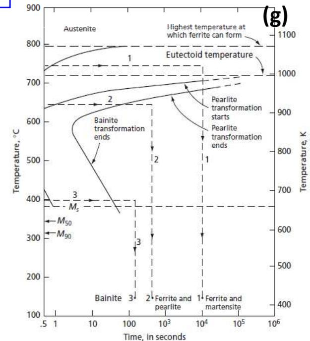
Fig. g: Arbitrary time-temperature paths on the isothermal diagram of a hypoeutectoid steel
