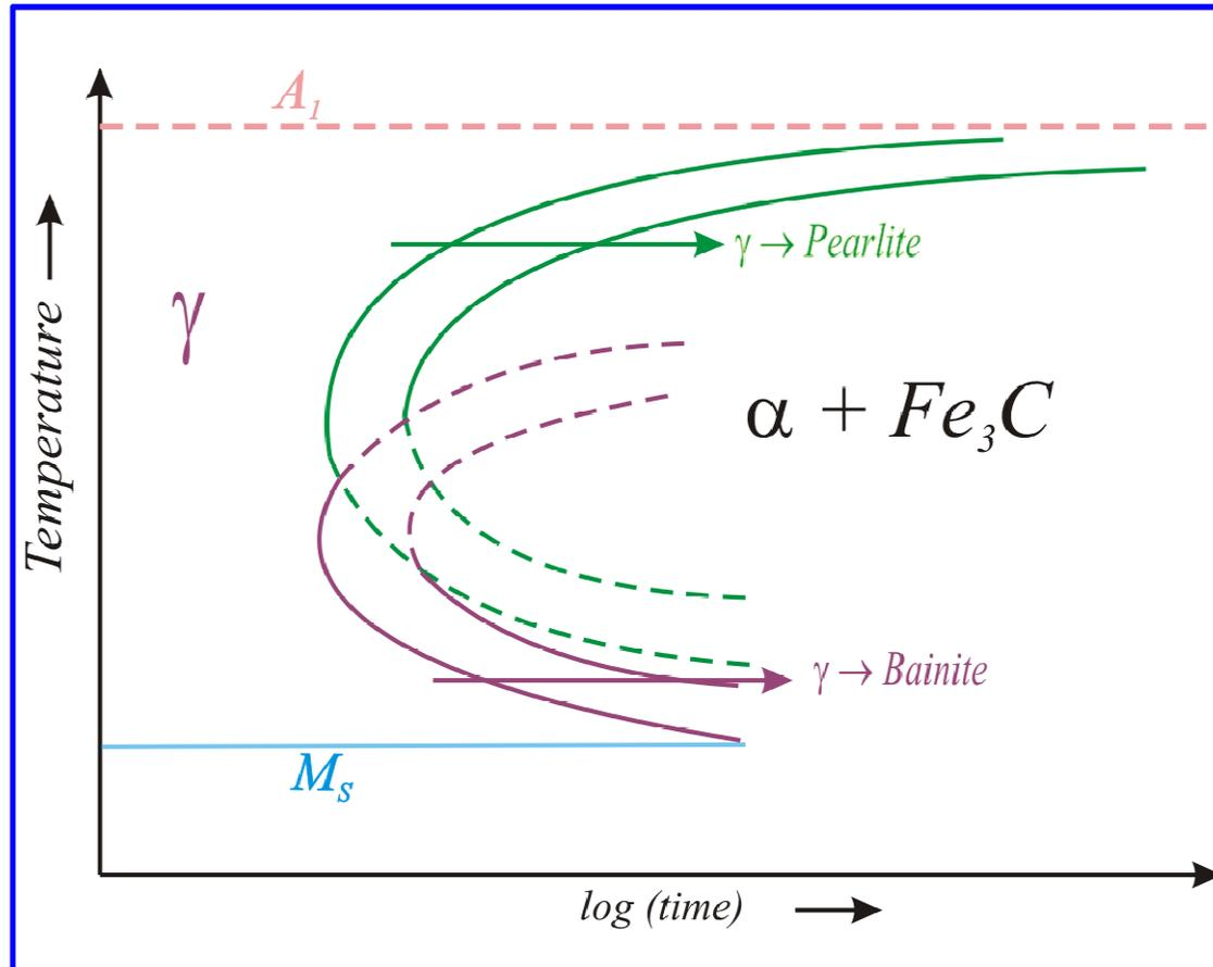
In principle two curves exist for Pearlitic and Bainitic transformations
