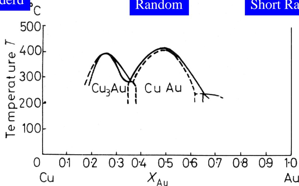
Part of the Cu-Au phase diagram showing the regions where the  $Cu_3Au$  and  $CuAu$  superlattices are stable.
