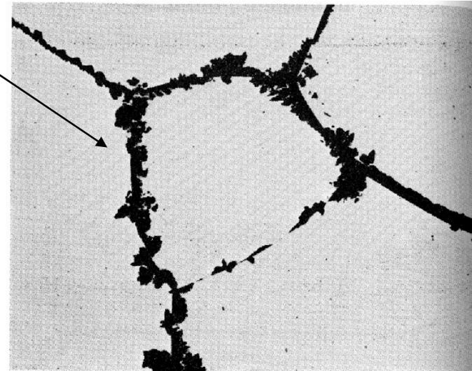
A partially transformed eutectoid steel. Pearlite has nucleated on grain boundaries and inclusions ( $\times 100$ ). (After J.W. Cahn and W.C. Hagel in *Decomposition of Austenite by Diffusional Processes*, V.F. Zackay and H.I. Aaronson (Eds.), 1962, by permission of The Metallurgical Society of AIME.)
