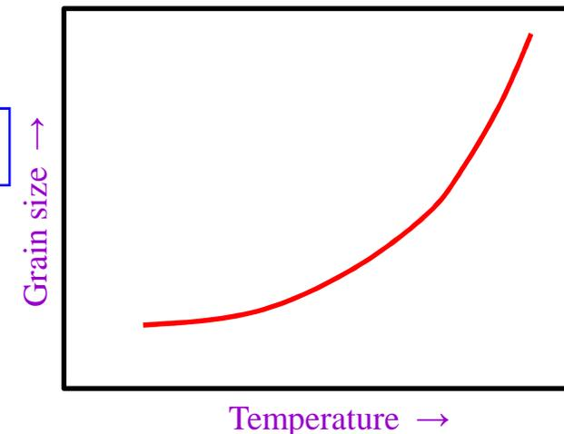
Effect of temperature on recrystallized grain size
