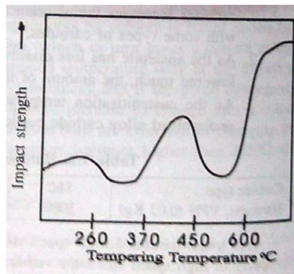
Schematic illustration of effect of tempering temperature on impact strength in steels prone to embrittlement during tempering.
