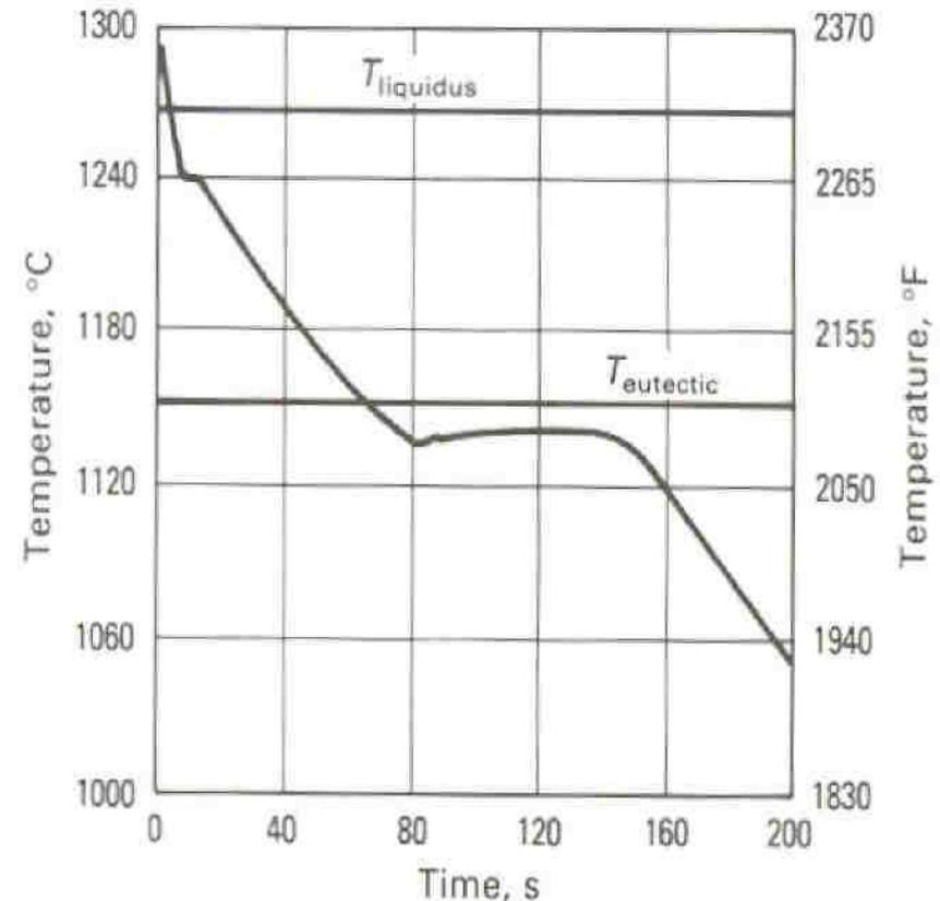
Cooling curve for an Iron-carbon alloy with 3.2% C. The solidification starts with a primary precipitation of austenite, followed by a eutectic temperature
