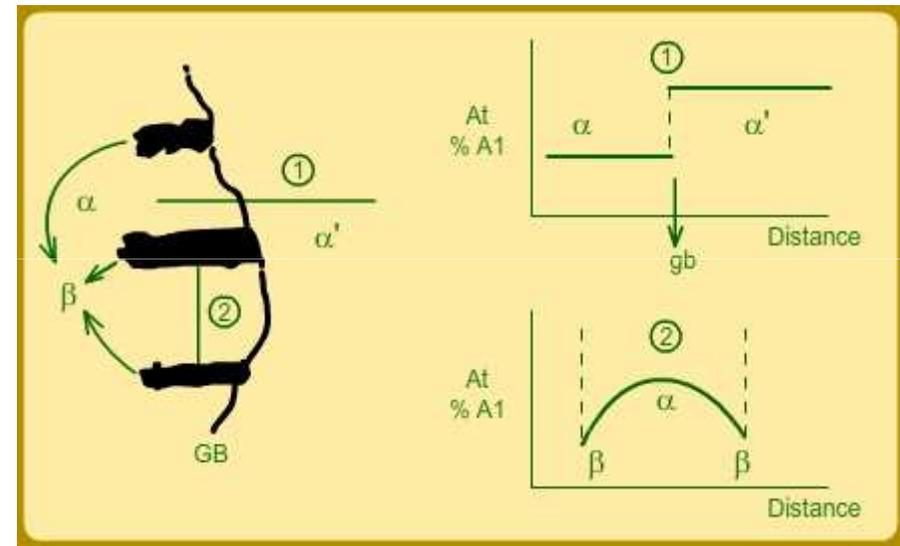
The cellular precipitation that takes place during the aging treatment leads to microstructures
