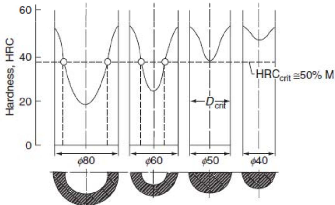
Determination of the critical diameter  $D_{crit}$  according to Grossmann
