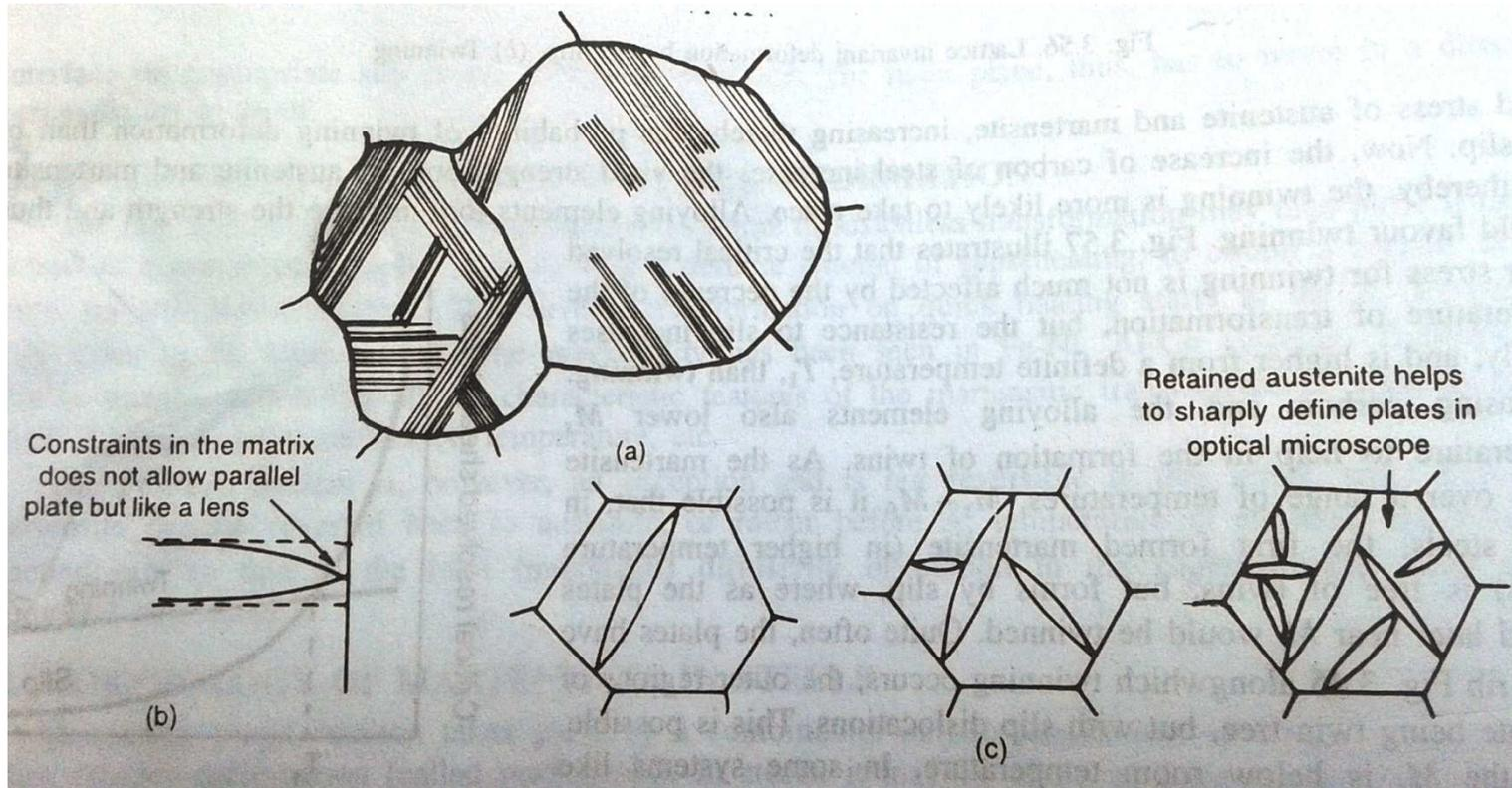
Formation of (a) Lath martensite (b), (c) plate martensite. (a) Schematic illustration of mode of nucleation and growth of lath martensite. (b) Lens Shaped martensite (c) Successive partitioning of austenite grain with the formation of plates of martensite
