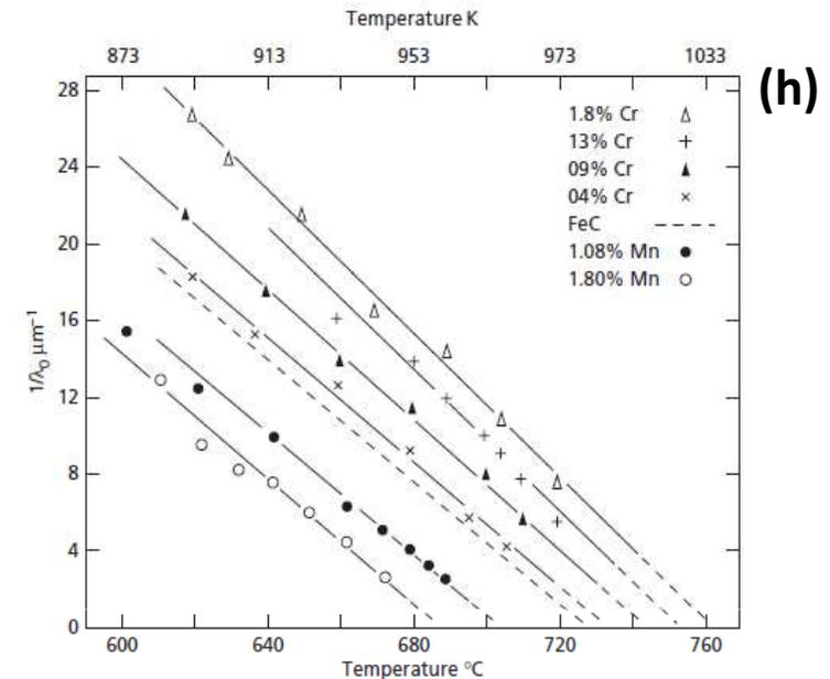
Fig. h: Minimum interlamellar spacing data for eutectoid steel containing additions of manganese and chromium
