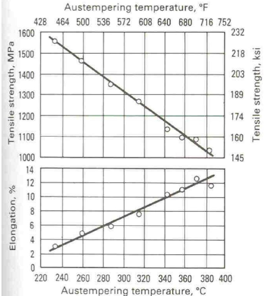
Relationship between austempering temperature and the strength and ductility of a 1.5Ni-0.3Mo alloyed ductile iron. Austenitizing temperature was 900°C.
