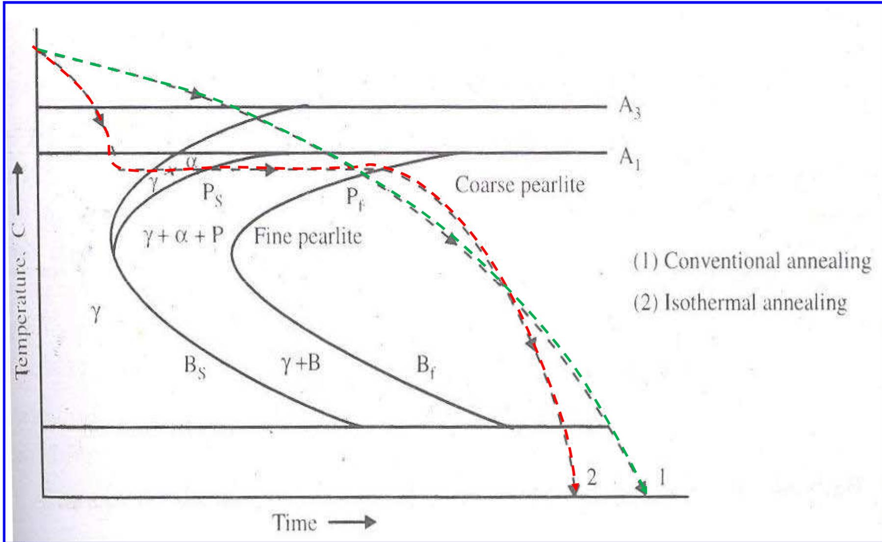
Isothermal annealing is primarily used for medium carbon, high carbon and some of the alloy steels to improve their machinability.
