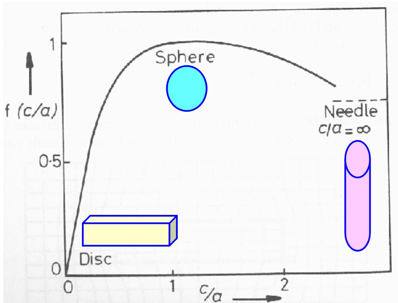
The variation of misfit strain energy with aspect ratio of ellipsoid shape
