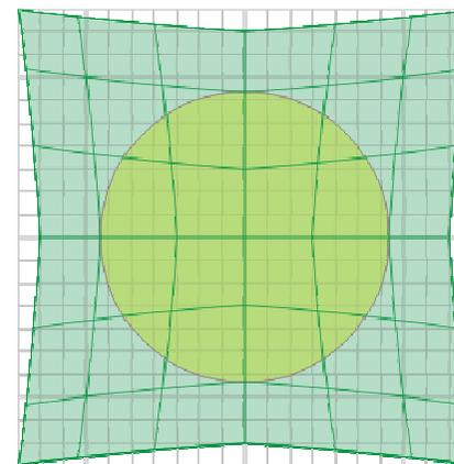
Schematic showing a coherent precipitate and the origin of coherency strains
