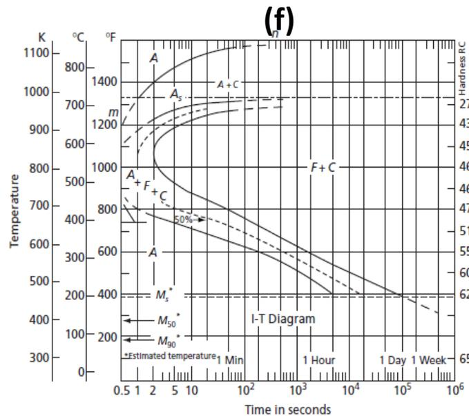
Fig. f: Isothermal transformation diagram for a hypereutectoid steel: 1.13 percent carbon, 0.30 percent manganese.
