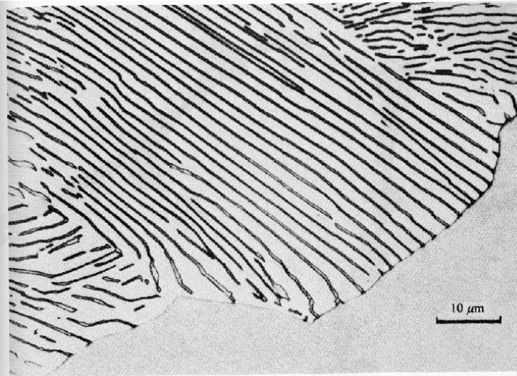
A pearlite colony advancing into an austenite grain. (After L.S. Darken and R.M. Fisher in *Decomposition of Austenite by Diffusional Processes*, V.F. Zackay and H.I. Aaronson (Eds.), by permission of The Metallurgical Society of AIME.)
