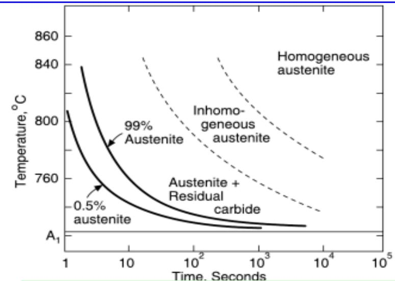
Effect of temperature and time on the austenite formed from pearlite in 0.3% carbon steel<sup>356</sup>
