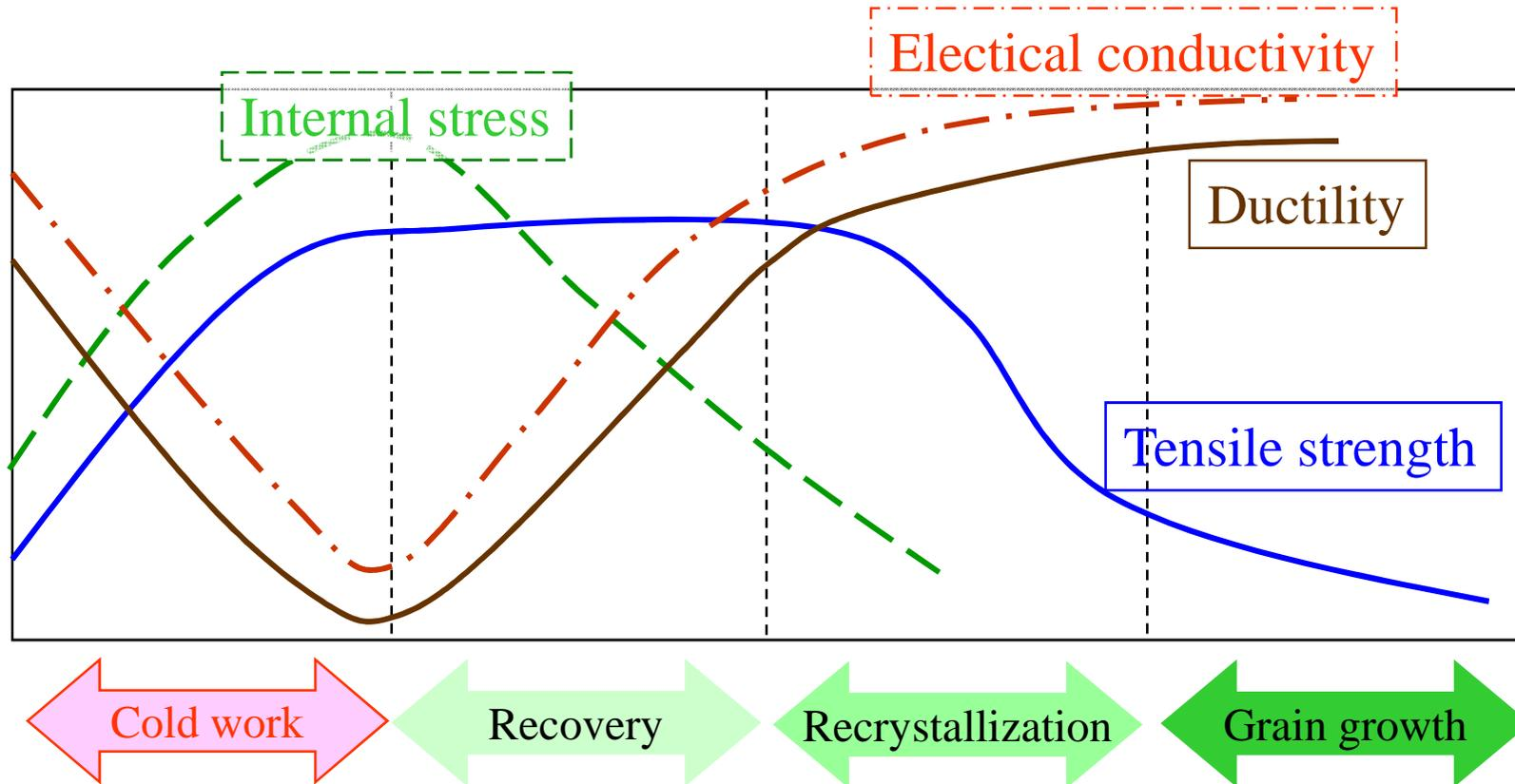
Change of properties with increased annealing temperature of a cold worked sample. Note that there are changes in properties beyond recrystallisation temperatures too due to grain growth.
