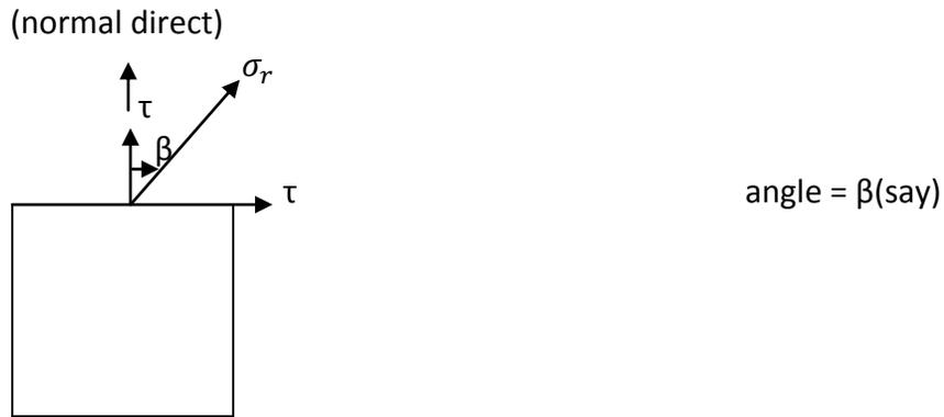
Suppose ' $\sigma_r$ ' is the resultant of normal stress ( $\sigma$ ) & shear ( $\tau$ ); & it makes an angle ' $\theta$ ' with the normal to the plane.
