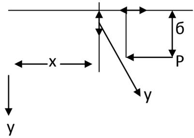
→ We Like to find out the minimum value of Load (P) for which the column is buckled.
