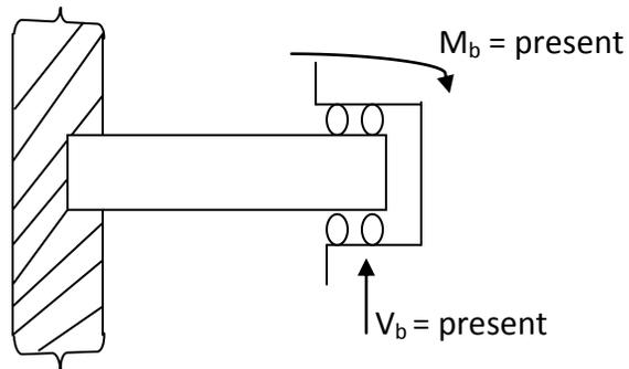
Shearing force :- of any section of a beam represents the tendency of the beam to one side of section to slide or shear laterally relative to other portion.
