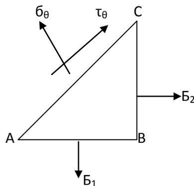
$$\sigma_\theta \times (AC \times t) = \left\{ \begin{aligned} &(\sigma_1 \times AC \times t) \times \sin \theta \\ &-(\sigma_2 \times BC \times t) \cos \theta \end{aligned} \right\}$$
