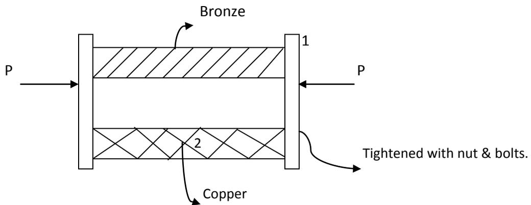
Both bars have same initial length & after deformation the two bars must remain together.
