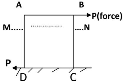
→ Apply a force (P) tangentially on the face of 'AB'. Then, there is a tendency for one part of body to slide over/shear from other part across any section 'MN'.
