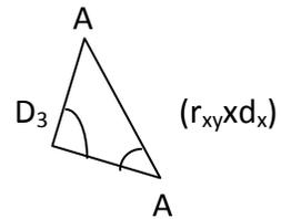
$$r_{xy\alpha} = \frac{(r_{xy} \times dx) \cos \alpha \cdot D_3 A}{ds}$$
