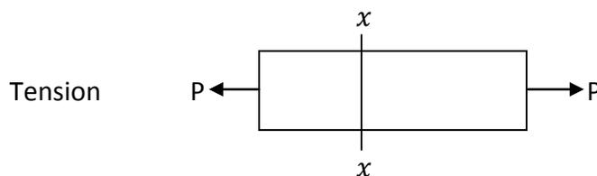
Ex Steel wire of a crane hook
