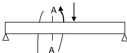
\*This refers to sagging bending moment because it tends to make the beam concave upward at section A-A.
