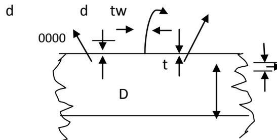
→ Replace the wire by an equivalent cylindrical shell of thickness 'tw'
