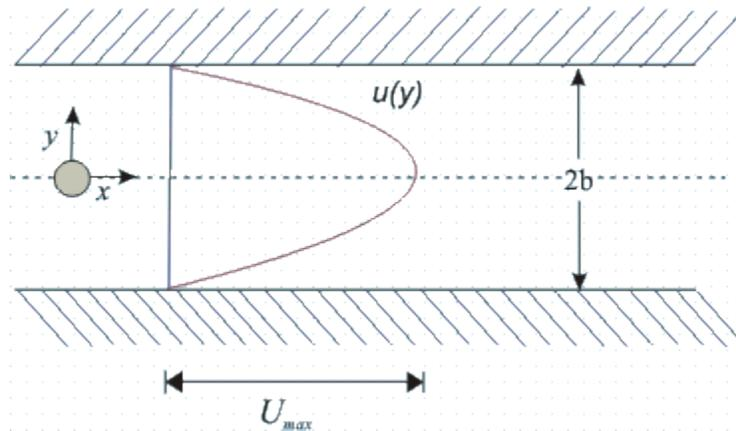
**FIG 25.2 Parallel flow in a straight channel**
