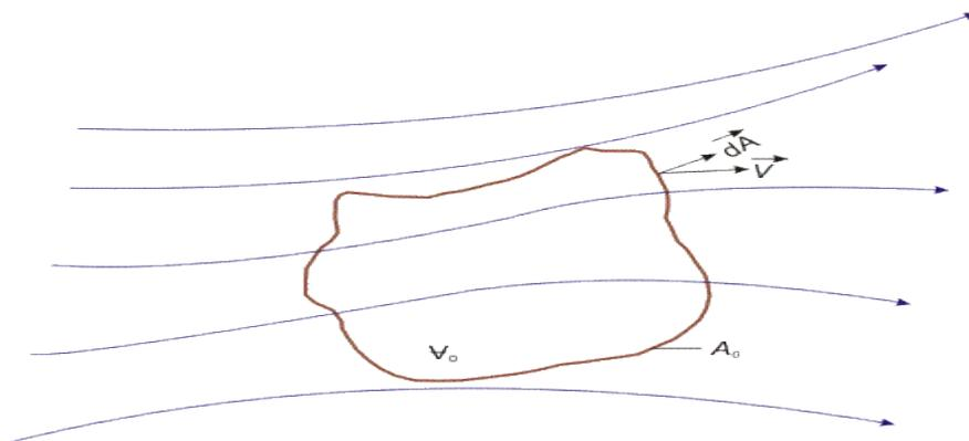
**FIG 25.1 Finite control volume fixed in space with the fluid moving through it**
