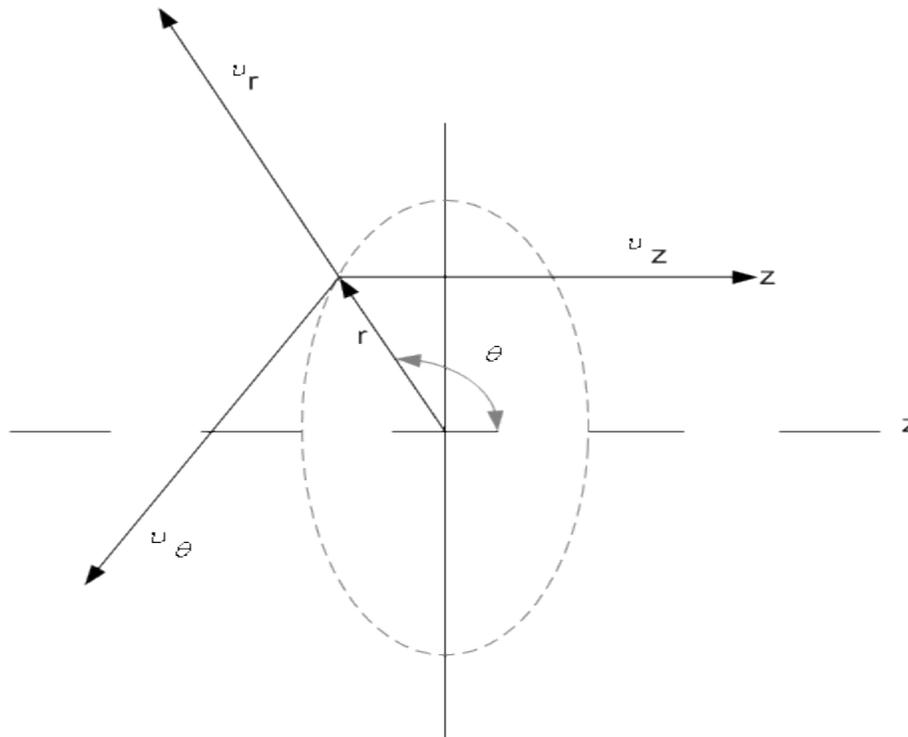
**FIG 2** Cylindrical polar coordinate and the velocity components
