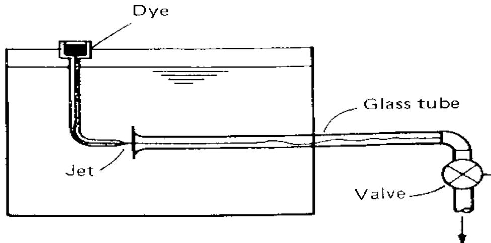
He used a tank arranged as above with a pipe taking water from the centre into which he injected a dye through a needle. After many experiments he saw that this expression
