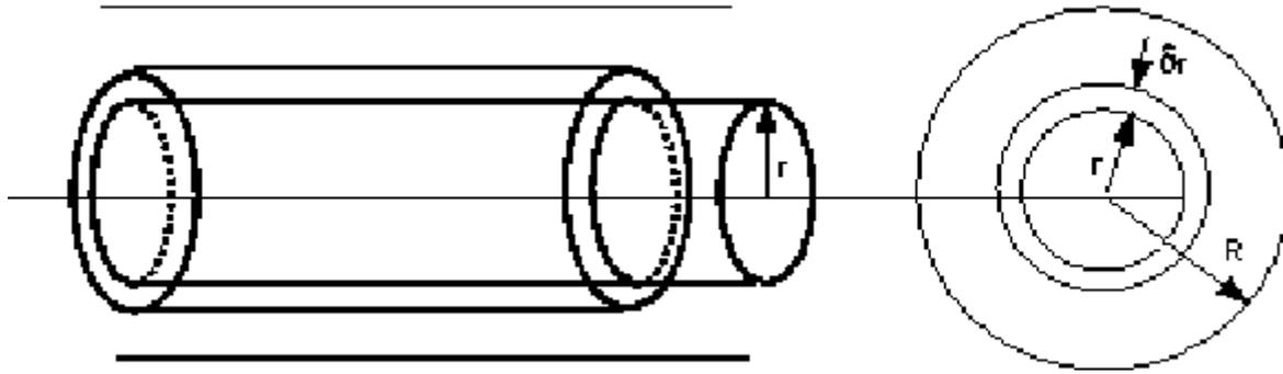
We are in equilibrium, so the shearing forces on the cylinder equal the pressure forces.
