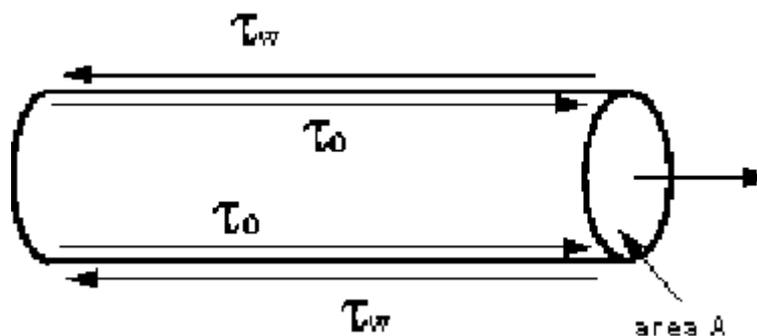
The pressure at the upstream end is  $p$ , and at the downstream end the pressure has fallen by  $\Delta p$  to  $(p - \Delta p)$ .
