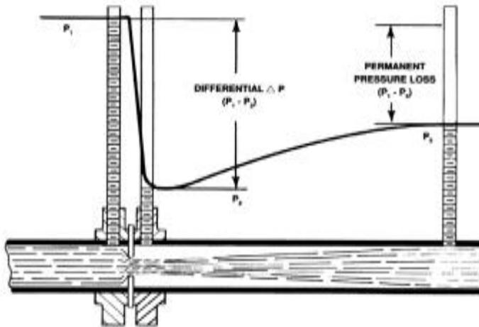
Typical Orifice Flow Pattern Flange Taps Shown
