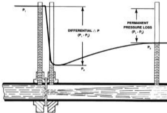
Typical Orifice Flow Pattern Flange Taps Shown
